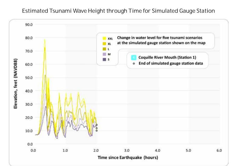
Figure 5: This chart depicts the tsunami waves as they arrive at the selected reference point (simulated gauge station). It shows the change in wave heights for all five tsunami scenarios over an 6-hour period. The starting water elevation (0.0 hour) takes into account the local land subsidence or uplift caused by the earthquake. Wave heights vary through time, and the first wave will not necessarily be the largest as waves interfere and reflect off local topography and bathymetry.
