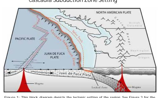
Figure 1: This block diagram depicts the tectonic setting of the region. See Figure 2 for the sequence of events that occur during a Cascadia Subduction Zone megathrust earthquake and
