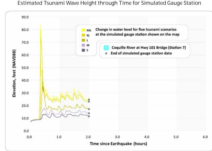
Figure 5: This chart depicts the tsunami waves as they arrive at the selected reference point (simulated gauge station). It shows the change in wave heights for all five tsunami scenarios over an 6-hour period. The starting water elevation (0.0 hour) takes into account the local land subsidence or uplift caused by the earthquake. Wave heights vary through time, and the first wave will not necessarily be the largest as
