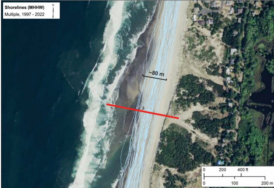
Figure 4-8. MHHW shorelines (blue lines) derived from repeat surveys of the beach for Transect 3 (red line) at Neskowin.
