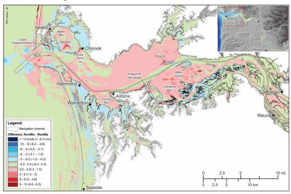
Figure 19. Maximum tsunami velocities (in knots) expressed as the difference between ebb slack (Run09a) and flood (Run06a) simulations, average river flow and friction. Velocities less than 0 indicate Run06a currents dominate, while velocities greater than 0 indicate that Run09a currents dominate.
