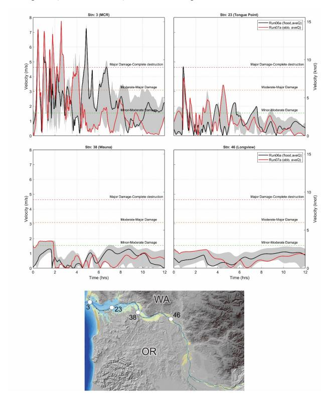
Figure 36. Time series showing the modeled currents generated for two simulations of a CSZ tsunami (L1) travelling along the navigation channel from the MCR to Longview. Gray shading denotes the envelope of variability in the tsunami currents from all simulations. Station 3 is at the mouth of the Columbia River, station 23 is at Tongue Point, station 38 is at Wauna, and station 46 is at Longview.
