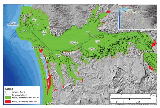
To highlight the upriver extent of the tsunami incursion associated with the maximum considered local event (Run05a), we define the maximum tsunami water level along the length of the navigation channel, which extends from offshore the mouth of the Columbia River (MCR) to Bonneville Dam (**Figure 15**). The maximum water level is defined as:
