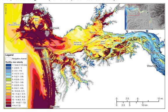
Comparisons between the two local events (XXL1 and L1) indicate large differences in the tsunami velocities along the Clatsop Plains, adjacent to the MCR, and in some isolated remote locations near the distal ends of the inundation zone (**Figure 13**). Upstream of Tongue Point, these differences drop to  $\sim 3$  knots or less.
