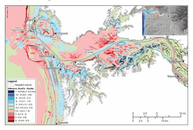
Figure 18. Maximum tsunami velocities (in knots) expressed as the difference between flood slack (Run08a) and flood (Run06a) simulations, average river flow and friction. Velocities less than 0 indicate Run06a currents dominate, while velocities greater than 0 indicate that Run08a currents dominate.
