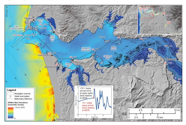
Figure 29. Maximum tsunami water levels interpolated along the Columbia River navigation channel for various AKMax simulations. Included in the plot are the expected wave arrival times. Blue shading denotes the range covered by high/low river flows, while gray shading covers the spectrum of responses associated with various tidal stages modeled using an average river flow.
