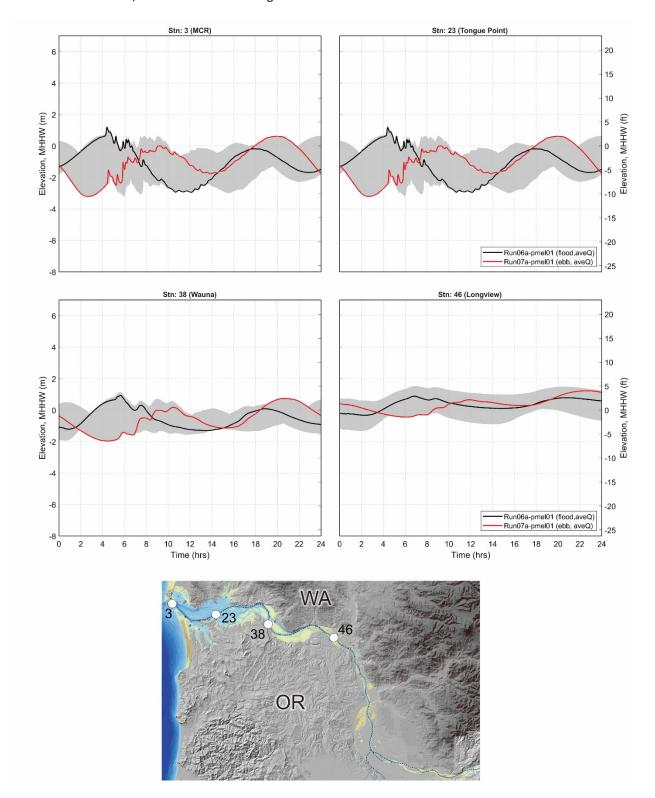
Figure 42. Time series showing the modeled currents for the AKMax tsunami traveling along the navigation channel from the MCR to Longview. Gray shading denotes the envelope of variability in the tsunami currents from all simulations. Station 3 is at the mouth of the Columbia River, station 23 is at Tongue Point, station 38 is at Wauna, and station 46 is at Longview.
