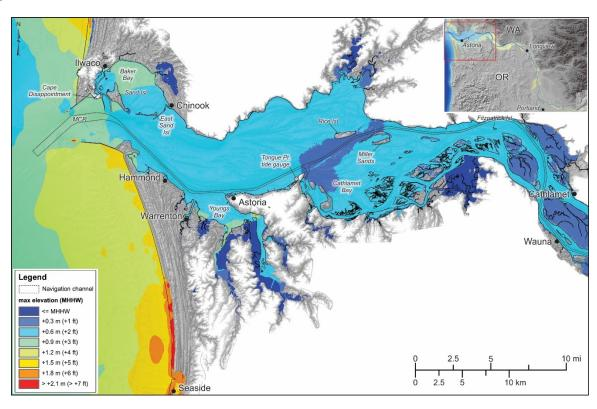
Figure 9. Simulated maximum water levels for the Alaska 1964 tsunami.
