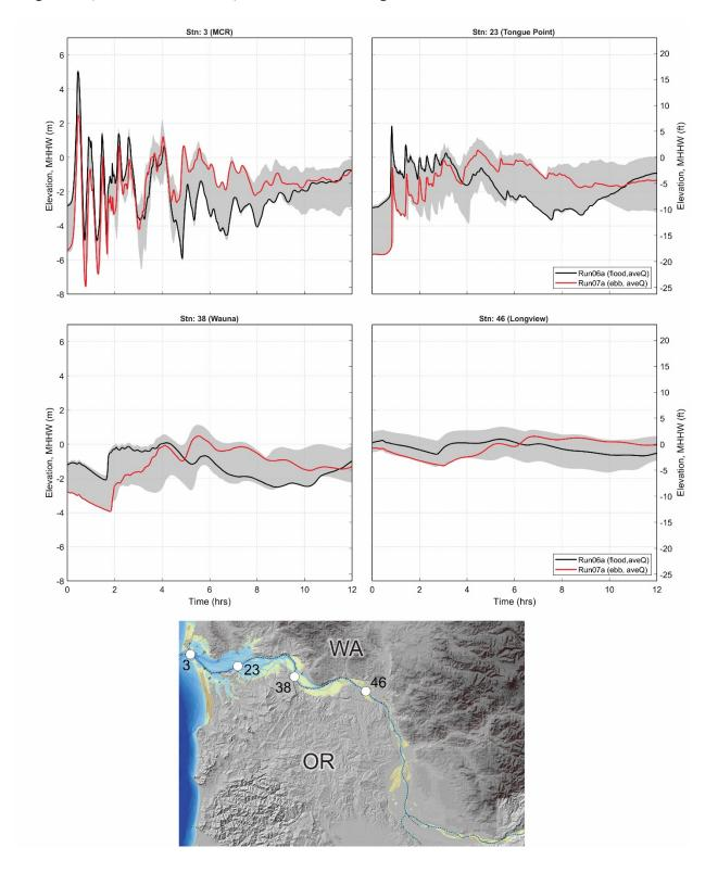
Figure 33. Time series showing the modeled water levels (flow depth—depth) for two simulations of a CSZ tsunami (L1) travelling along the navigation channel from the MCR to Longview. Gray shading denotes the envelope of variability in the water levels from all simulations. Station 3 is at the mouth of the Columbia River, station 23 is at Tongue Point, station 38 is at Wauna, and station 46 is at Longview.
