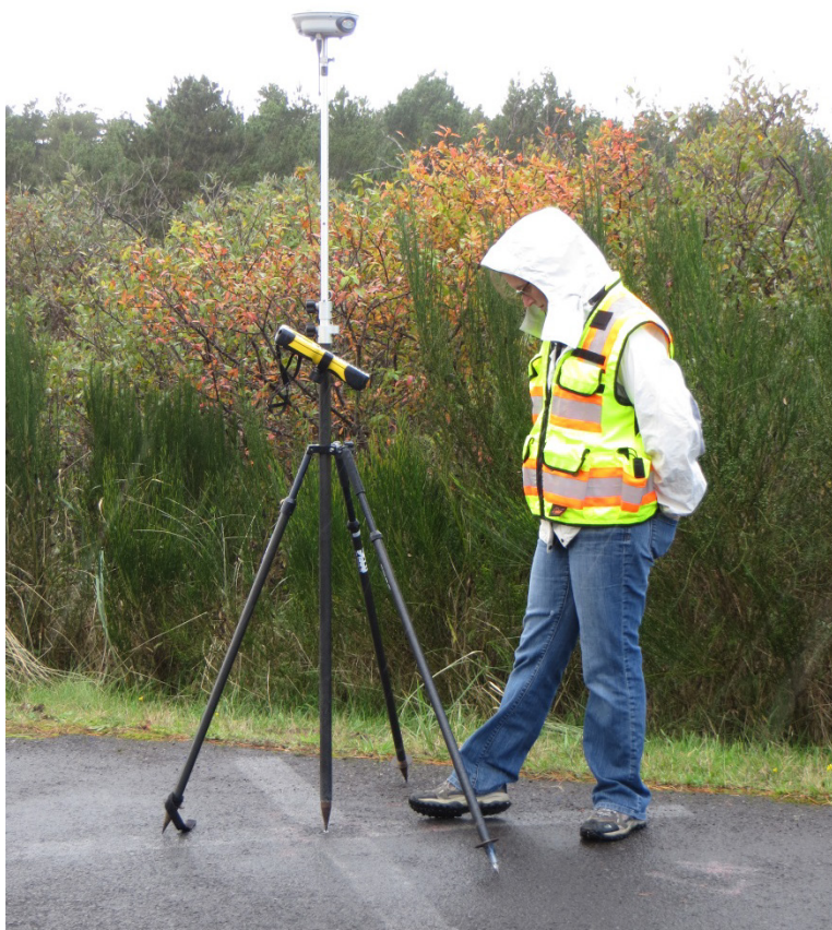
Figure 27. A 180-epoch calibration check is performed on a survey monument. This procedure is important for bringing the survey into a local coordinate system and for reducing errors associated with the GPS survey. (Photo credit: J. Allan, DOGAMI)
