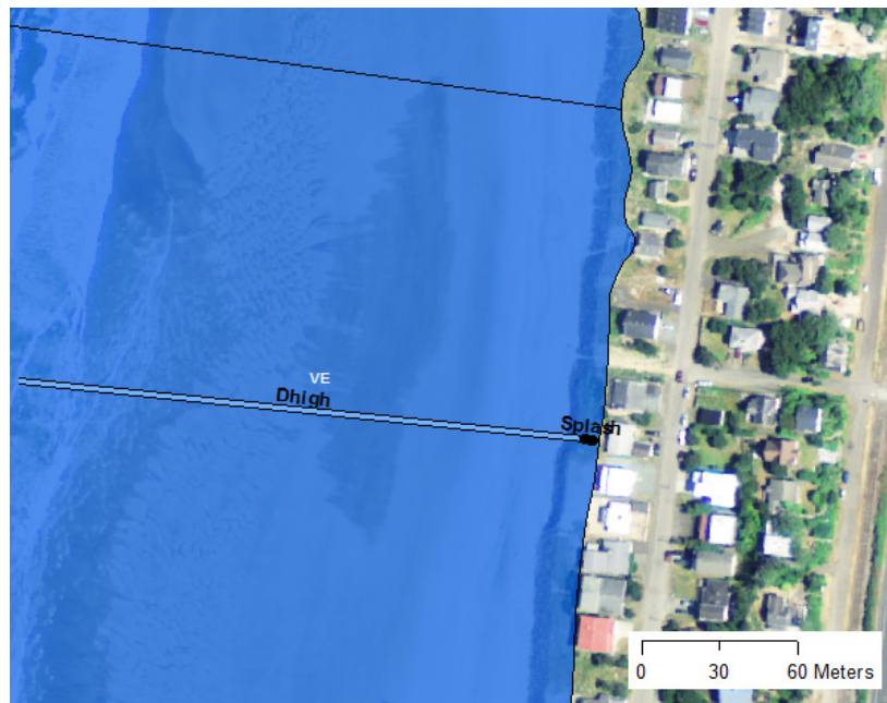
Figure 8-4. TILL 144 transect at Rockaway with overtopping splash zone. The short splash zone distance (black) was added to the extent of the VE zone.
