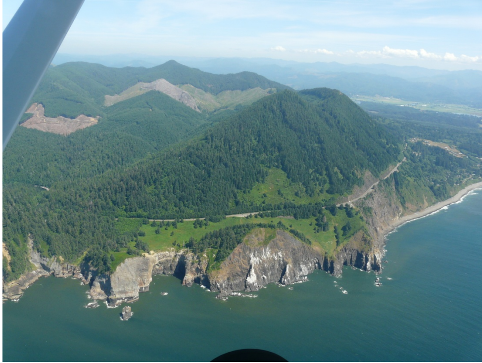
Figure 2-2. Looking east at Neahkahnie Mountain. U.S. Highway 101 can be seen around mid photo tracking along the mountain. To the right and along the toe of the bluff is an extensive cobbles/boulder berm that has formed as a result of rockfalls and landslides off the headland (photo: L. Stimely, DOGAMI, 2011).
