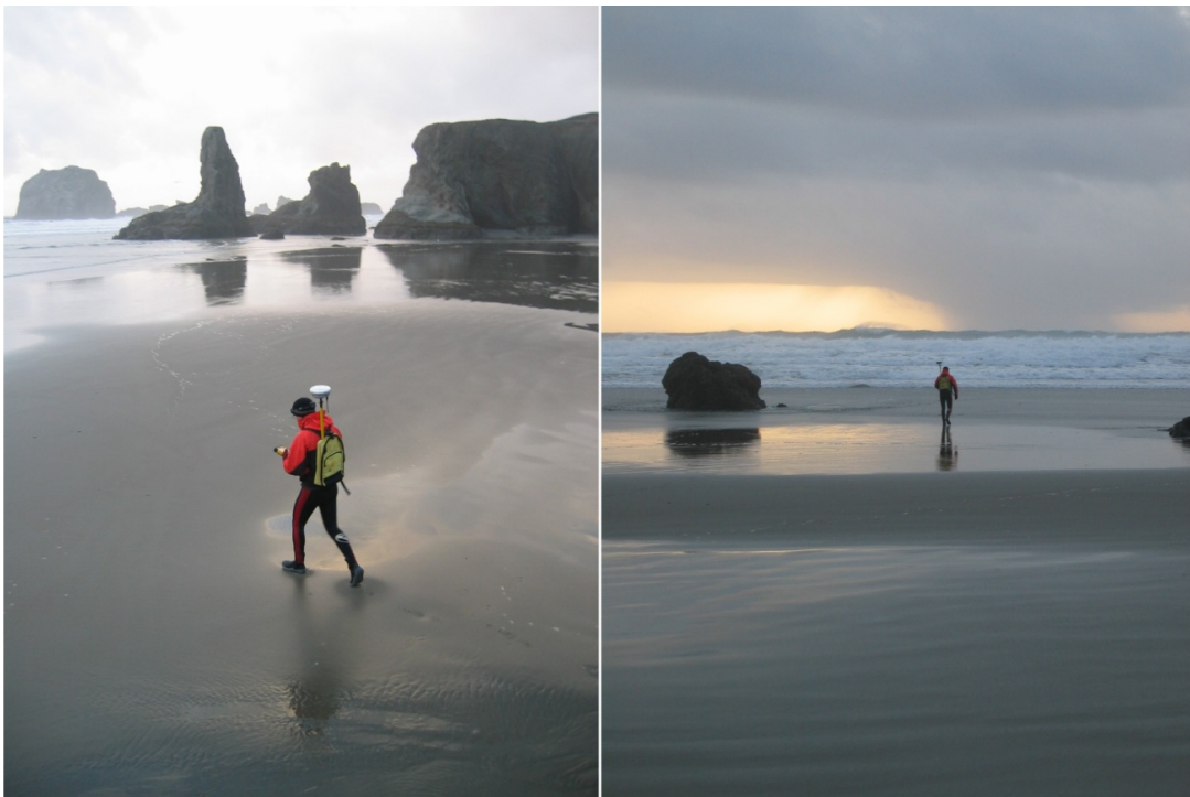
Figure 3-6. Surveying the morphology of the beach at Bandon using a Trimble 5800 “rover” GPS (photo: J. Allan, DOGAMI, 2009).
