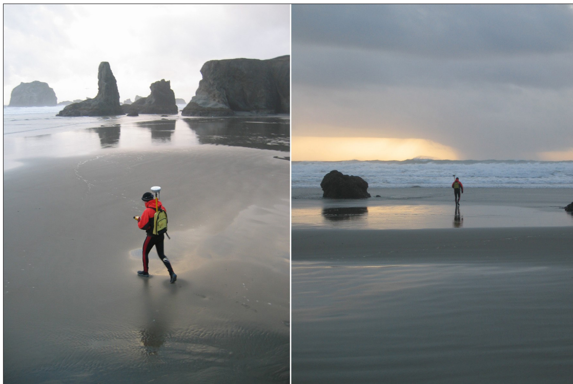
Figure 3-4. Surveying the morphology of the beach at Bandon using a Trimble® 5800 “rover” GPS.
