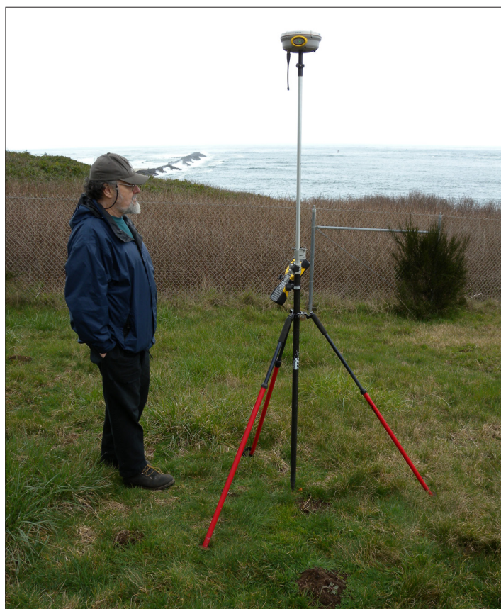
Figure 3-3. A 180-epoch calibration check is performed on a survey monument (OLC5PGW1) established by WS near the Coast Guard observation tower at the mouth of Coos Bay. This procedure is important for bringing the survey into a local coordinate system and for reducing errors associated with the GPS survey.
