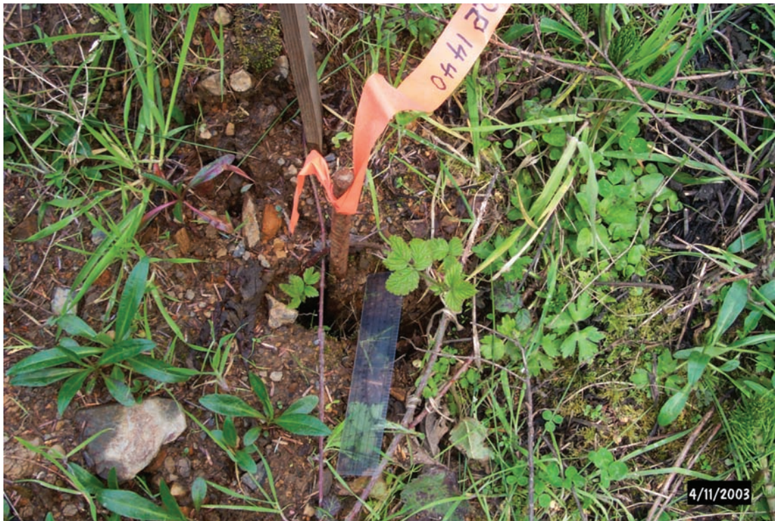
Figure G6. Marker nail site JC-17 with displaced steel survey marker at headscarp, looking east. This stake was not used in the resurvey.
