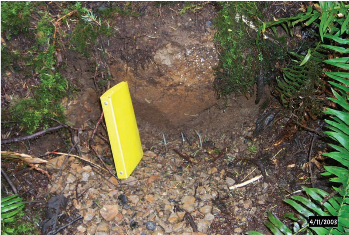
Figure G9. Marker nail site JC-19 looking south. Yellow field book is ~19 cm long. Note that all nail heads are still touching in this April 2003 photograph, so no significant movement occurred. Scarp is in relatively fresh Astoria Formation siltstone and sandstone with a thin covering of gravel from the Old Coast Highway.
