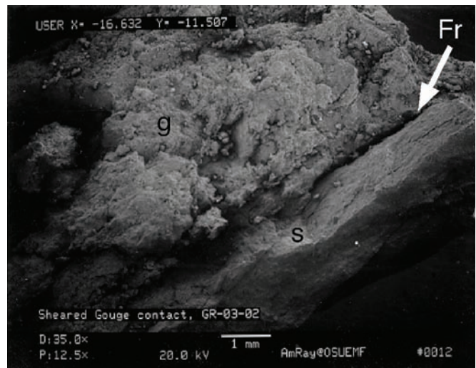
Figure A5b. SEM photomicrograph at low magnification (12.5x) shows a sharp smooth shear plane (labeled Fr) that appears to step across the specimen. The specimen was mounted upside-down, which places the shear gouge (g) in the upper NW half of the photograph and the unsheared siltstone (s) in the lower SE half of the photograph. The sheared gouge appears as a jumbled mass of largely subparallel (imbricated) smectite clay particles or packets. In the gouge, multiple fractures (dark lines), along which slippage has occurred, are subparallel the main shear boundary.
