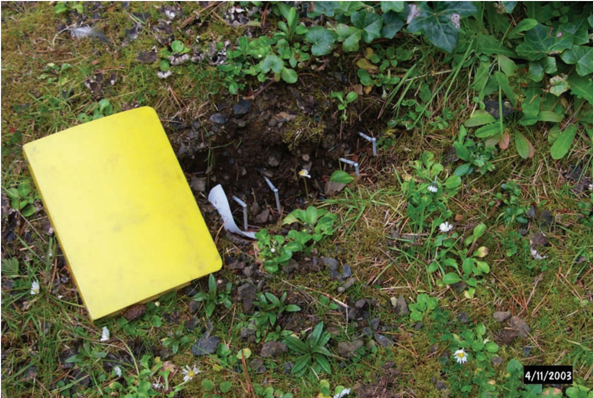
Figure G16. Marker nail site JC-23 on north margin of the landslide looking east southeast. Yellow field book is ~19 cm long.
