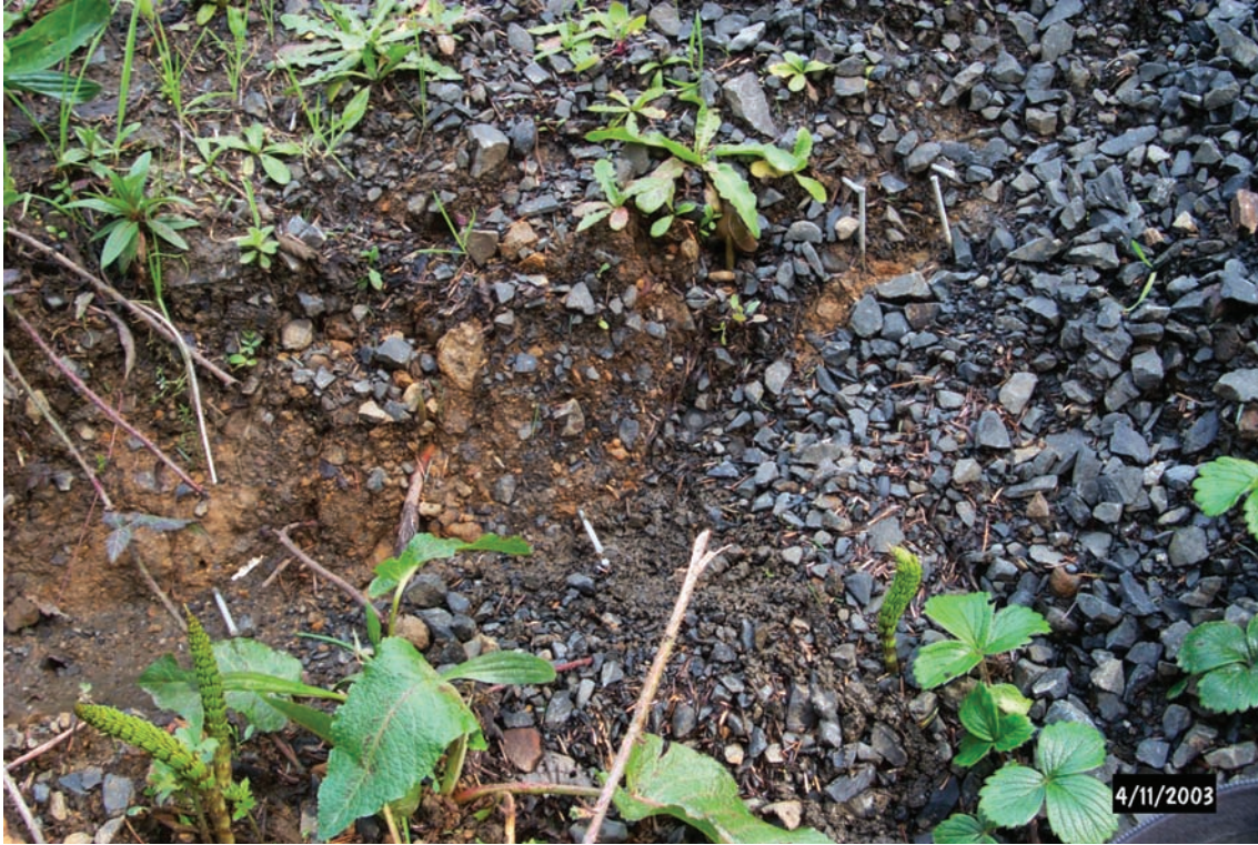
Figure G8. Marker nail site JC-18, looking southeast. The scarp is in gravel fill from the forest road. Exposed portions of the two vertical nails on the right are ~1.2 cm long. Note that fresh gravel dumped on the road has disturbed the nails on the right, so that measurement was not used.
