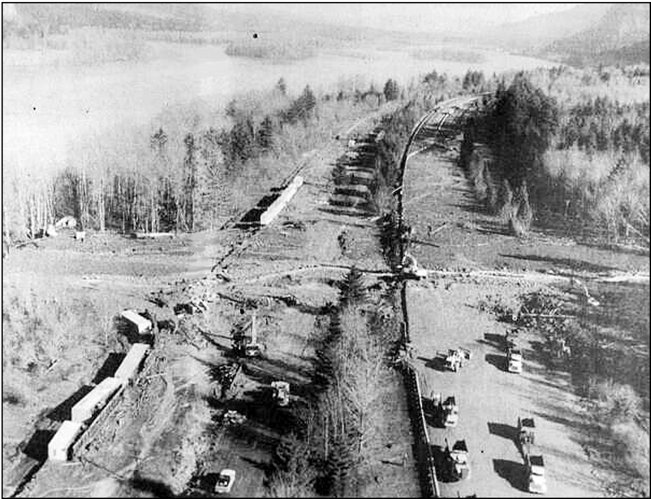
Figure 6. The Tumalt Creek Debris Flow looking east. Note the destruction on Interstate 84 and the Union Pacific Railroad (courtesy of The Oregonian).
