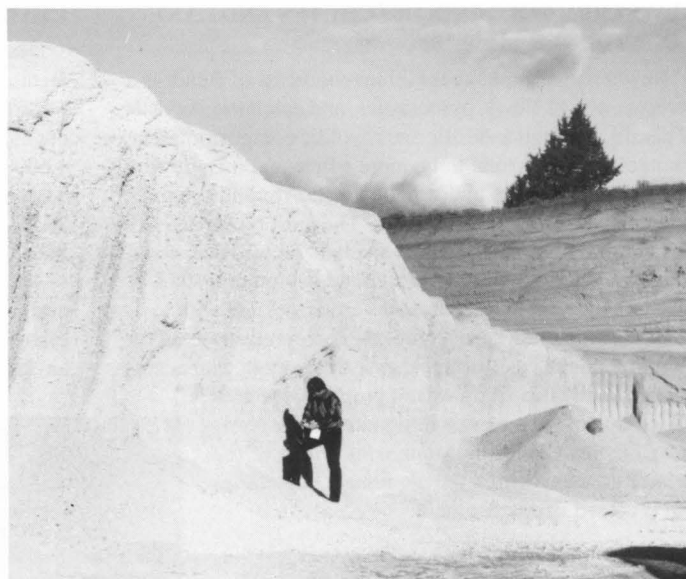
Figure 17. Cascade Pumice Company pit in Bend pumice unit near Tumalo, Deschutes County. Overlying Tumalo tuff, visible in background, has been removed just prior to mining pumice.
