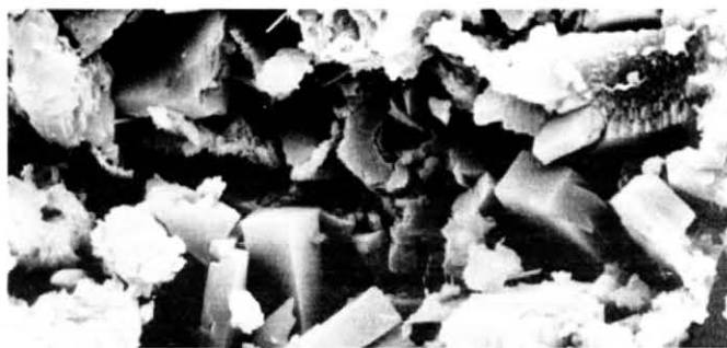
Figure 11. SEM image of Harney Basin mixed chabazite/clinoptilolite with minor montmorillonite, Oregon.
