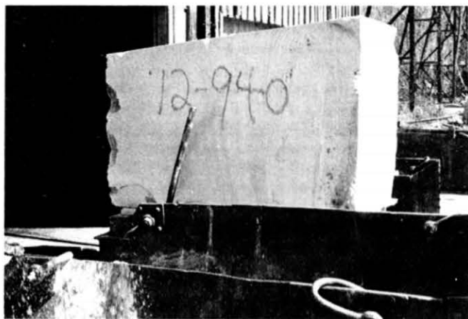
Figure 7. Soapstone block ready to be slabbled with a Tysaman sand gangsaw, The New Alberene Stone Company, Schuyler, Nelson County.
