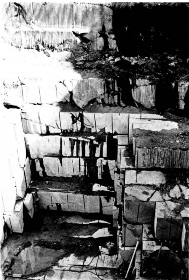
Figure 6. Quarry showing vertical drill holes at the top and smooth surfaces below of stone cut with a Korfmann chain saw, The New Alberene Stone Company, Schuyler, Nelson County.
