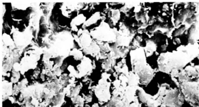
Figure 20. SEM image of "Robin's Egg Blue" clinoptilolite, northern Washakie Basin, Wyoming. Note that clinoptilolite crystals are highly etched.
