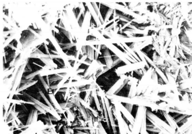
Figure 13. SEM image of erionite from "Billboard Cliffs" area, Rome district, Oregon. Letter "E" indicates typical acicular erionite crystal.
