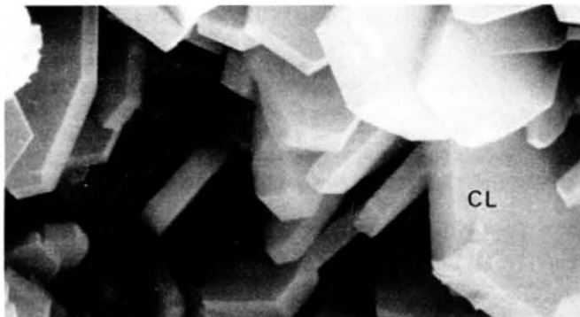
Figure 21. SEM image of "Robin's Egg Blue" clinoptilolite. Letters "CL" indicate large, euhedral, unetched clinoptilolite crystal.
