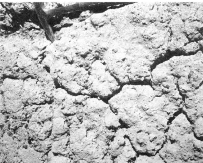
Figure 12. Alligator-hide weathering of bentonite.
