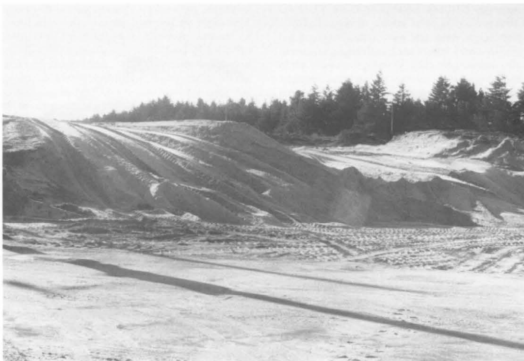
Figure 1. CooSand Corporation in North Bend, Coos County. Quartzofeldspathic dune sand is mined by front end loader and shipped by rail to Portland for production of colored glass containers.
