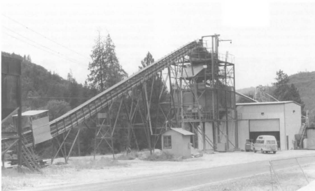
Figure 5. A portion of the Bristol Silica and Limestone Company processing plant where crushed quartz from the pit is further crushed, screened, and bagged.
