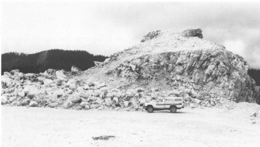
Figure 3. Quartz Mountain, Douglas County. Quartz replacement body is mined, crushed, and screened on site and shipped by truck to Riddle, Oregon, for use in nickel smelting and ferrosilicon production.
