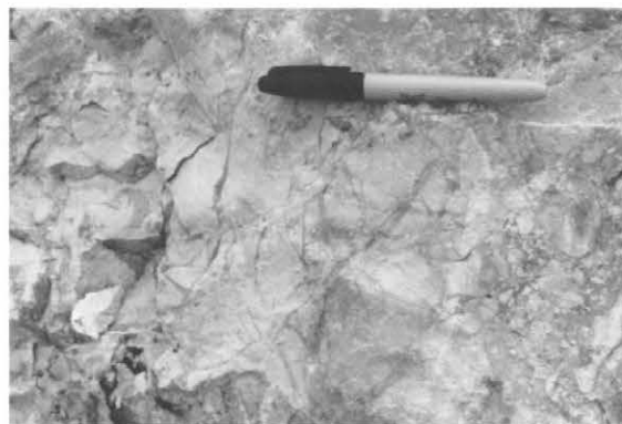
Figure 2. Relict volcanic texture in quartz replacement body of the Quartz Mountain deposit, Douglas County.
