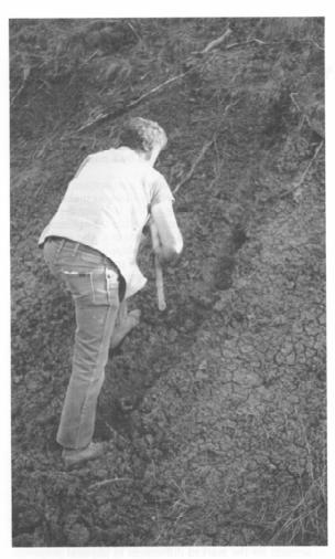
Figure 9. Shallow sample trenching of bentonite outcrop at site 12.
