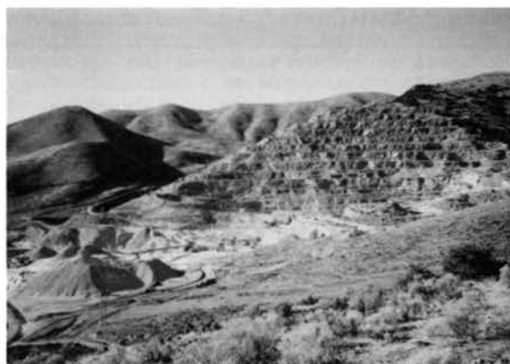
Figure 12. Durkee quarry (locality F-6) and stockpiles. Primary crusher and screening facility in middle ground. Stockpiles to left are screened sugar rock in front and cement rock in rear.
