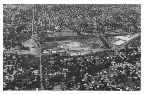
Figure 12b. Some site being developed for industrial park. Note how highwalls have been shaped for public safety.
