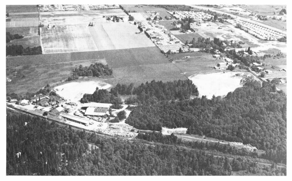
Figure 2. Oblique aerial view of Multnomah County site 44 showing Columbia Brick Works, Inc. Note that pit is being mined on slope, which allows easy reclamation.
