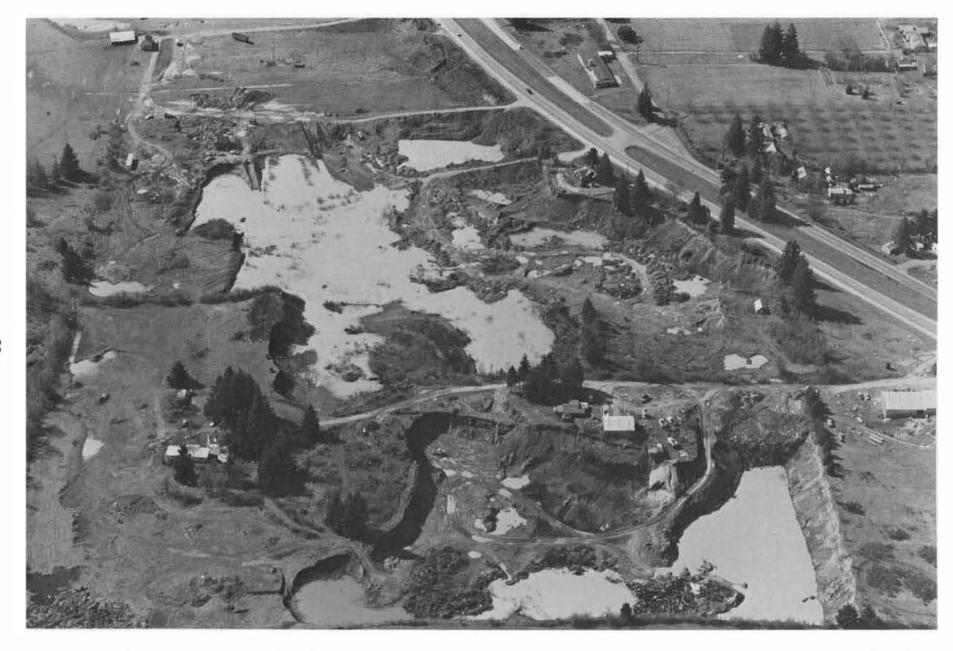
Figure 10. Oblique aerial view of Washington County sand sites 41 and 43 showing water and highwall ground-support hazards.
