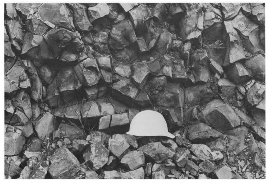
Figure 6b. Close-up view shows fins jointing size (1-6 in.) of basalt, which can be mined by ripping.
