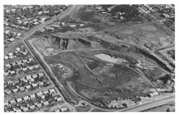
Figure 13a. Oblique aerial view of Multnomah County site 16 showing resource nearly depleted and demolition filling begin.
