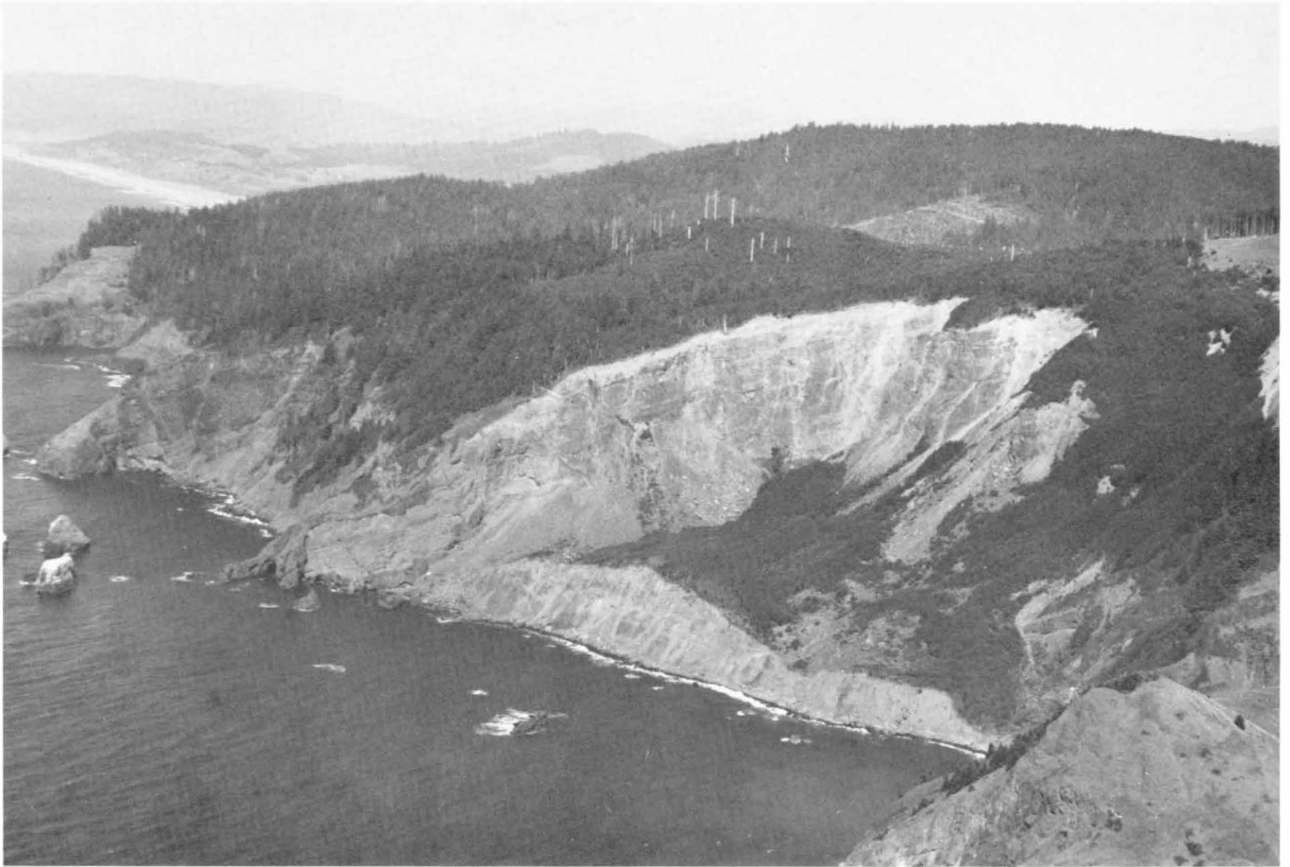
Figure 5. Deep bedrock slide which destroyed 20 acres at Cascade Head is the result of coastal erosion and a unique distribution of geologic units with varying engineering properties. Geologic investigations are needed to outline areas of potential future hazard.
