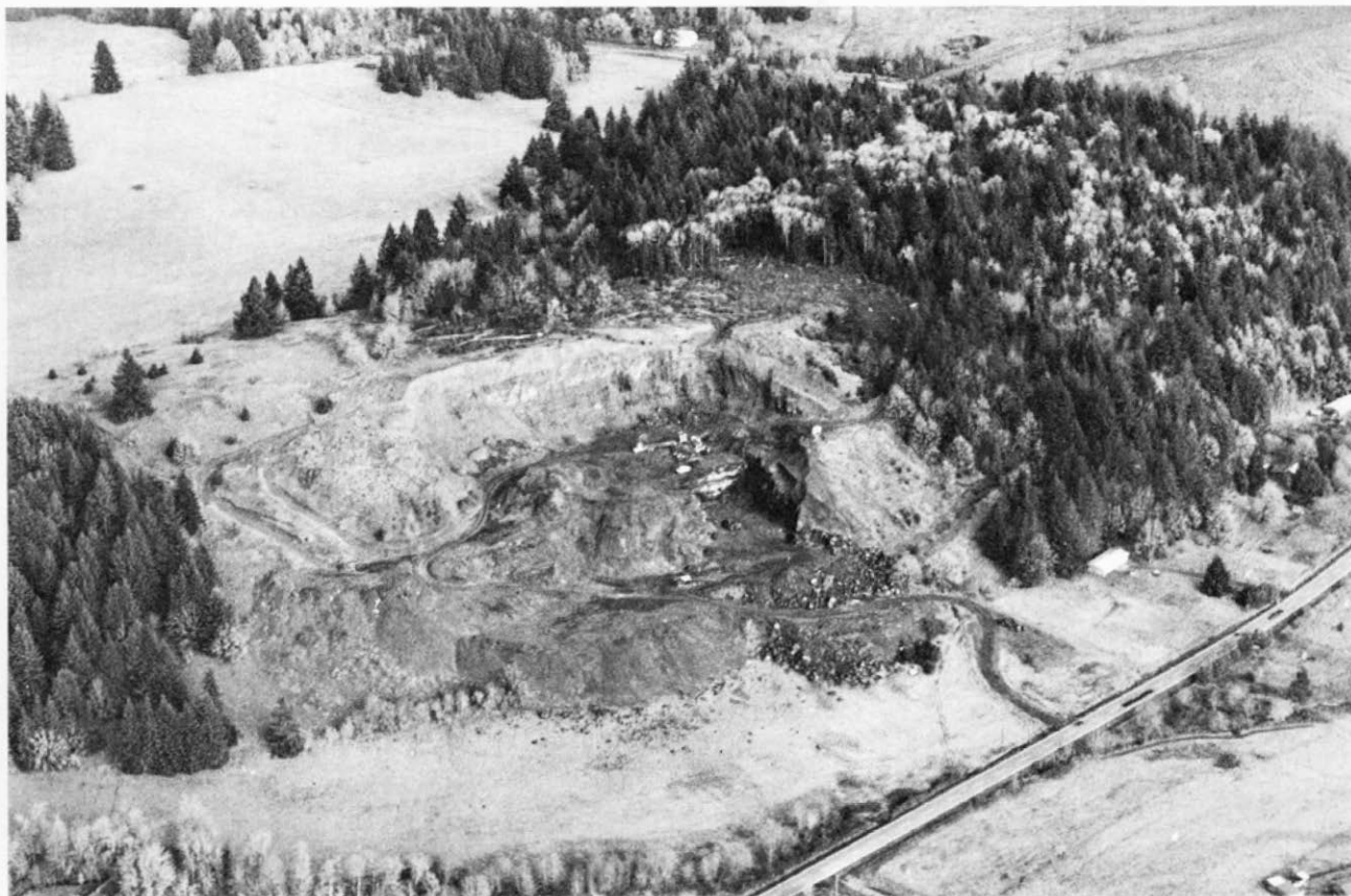
Figure 3. Oblique aerial view of quarry site 33 at Wren. Quarry has been developed in massively jointed Siletz River Volcanics. As quarrying has gone deeper into the ridge, overburden has become greater and jointing more widely spaced, producing more massive rock fragments. This site cannot be screened from view of State Highway 20.
