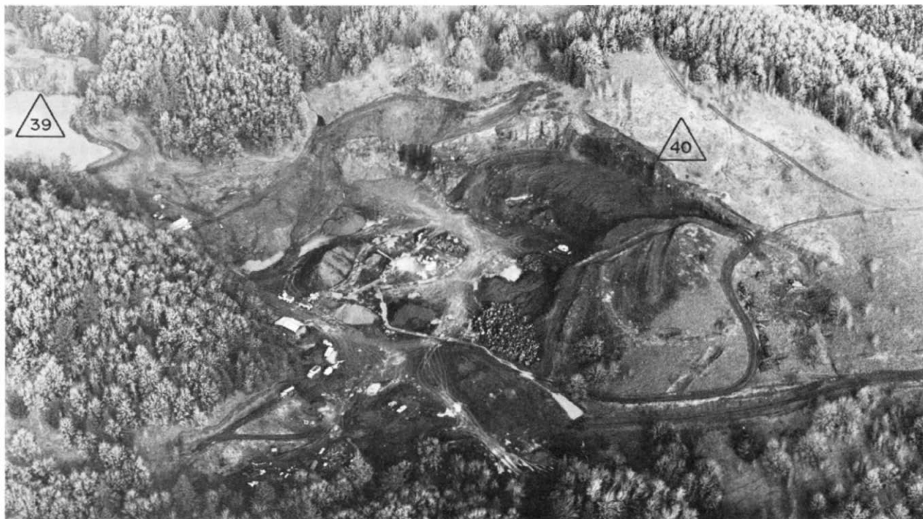
Figure 6. Oblique aerial view of sites 39 and 40. Site 39 is hazardous because it has steep walls and is water filled. Site 40 demonstrates current mining practices: top of ridge instead of bottom of slope is being mined; other benches are started as needed to keep highwalls at workable heights. Access to both sites is controlled, and neither can be seen from any public road.
