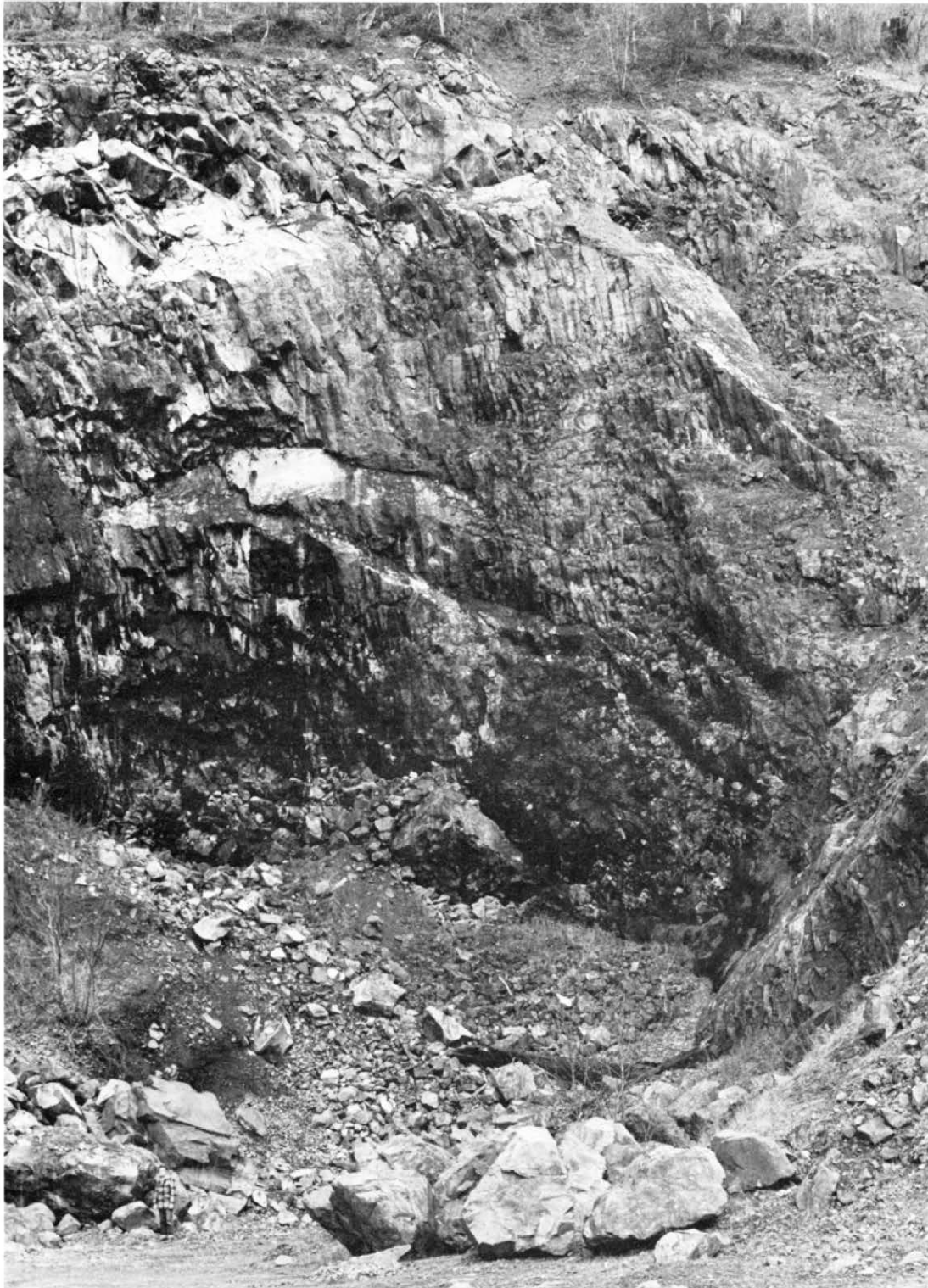
Figure 5b. Site 123. Note man in foreground for scale. Hazards include highwall heights, large loose boulders on sloping fracture planes, and loose overburden at top of quarry.
