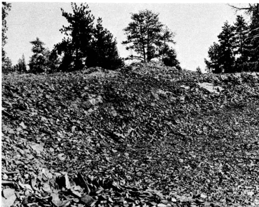
Photo 10. Platy basalt quarried by U.S. Forest Service (No.223) in sec. 36, T. 45 S., R. 33 1/2 E. Pit-run rock (uncrushed) is suitable for base rock. A small crusher is adequate to produce crushed rock from this material.
