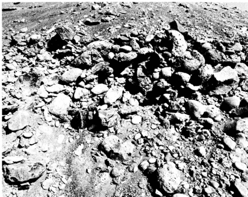
Photo 12. Close-up view of fluvioglacial gravel at Umatilla (No. 48). The gravel is composed of rounded to subangular stones ranging in size from sand to cobbles and composed of dense to vesicular basalt. Selective excavation is used to produce the desired gravel gradation.
