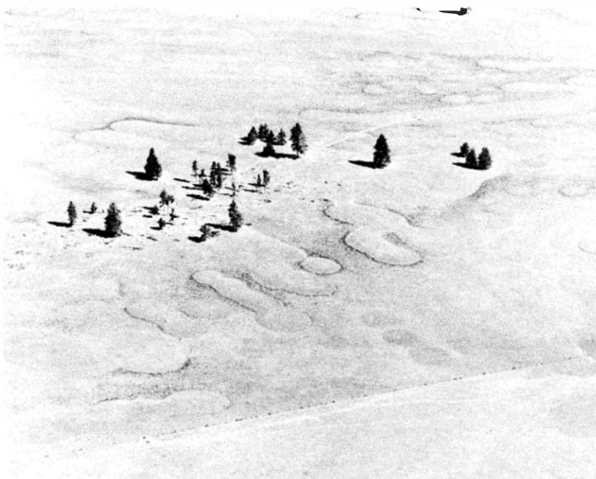
Photo 9. Rock patterns on surface indicate very thin soil cover over basalt bedrock. Good rock quarries can be located where access and topography are favorable for a crushing plant.
