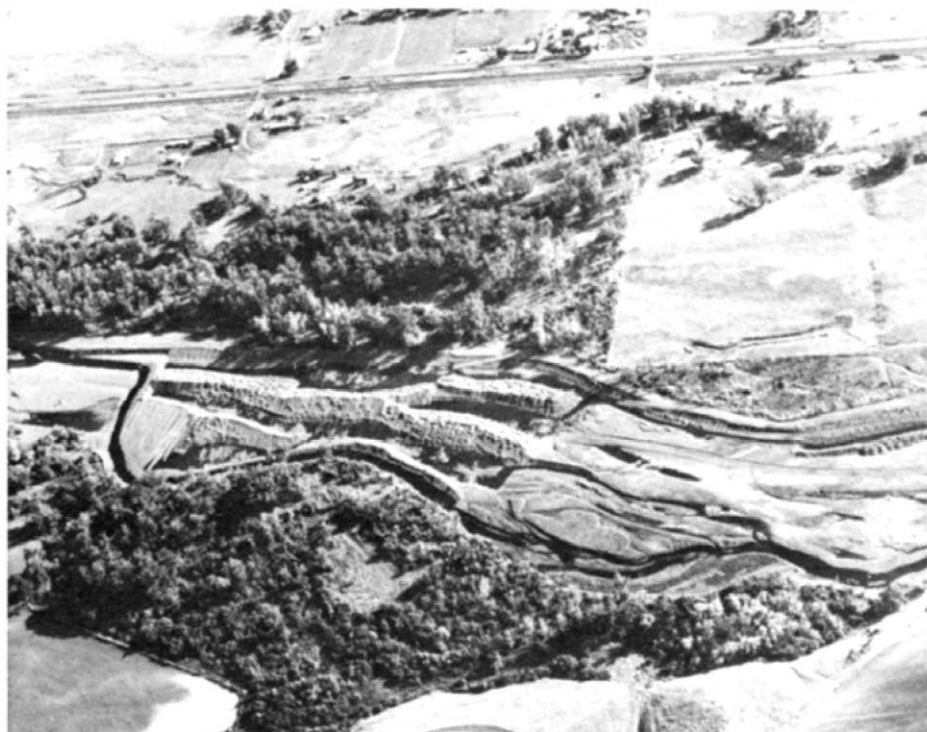
Photo 6. Commercial gravel for use at Pendleton is produced on the Indian Reservation at Mission (site No. 145). The gravels are replenished by occasional floods where stream gradient is decreased.
