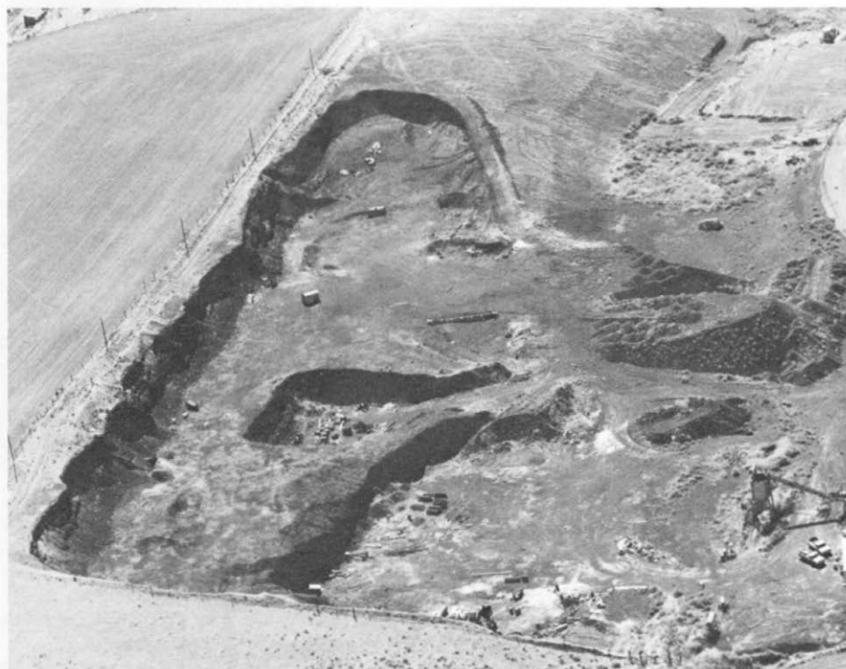
Photo 14. Jellum quarry (No. 151) in Columbia River Basalt just southeast of Pendleton Airport. Steep quarry faces adjacent to property lines will make reclamation difficult.
