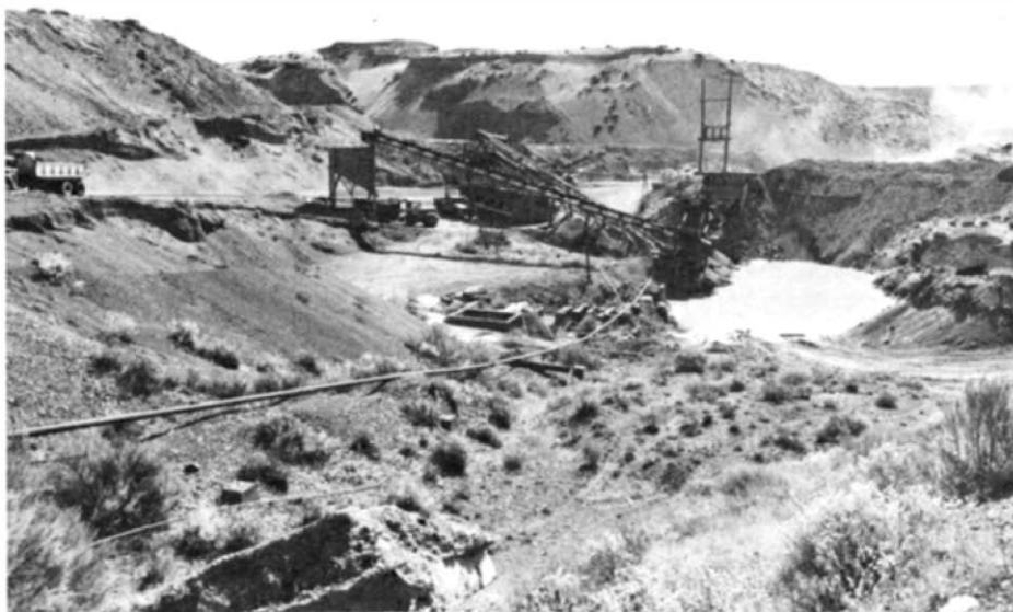
Photo 5. Jones-Scott Company produces gravel commercially at Umatilla from this pit (No. 46) just southeast of the city. Fluvioglacial deposits vary from cross-bedded sand to gravel.
