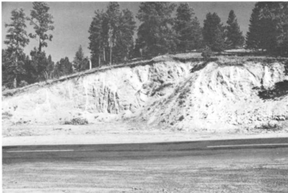
Photo 7. Granite quarry (No. 218) near Battle Mountain. The granite has disintegrated to individual grains.
