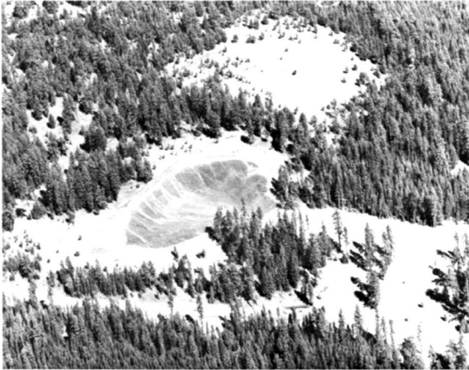
Photo 3. Small quarry (No. 233) in Umatilla National Forest. Sloping walls are safety feature to protect animals and vehicles.
