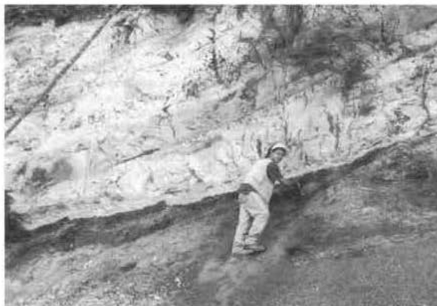
Figure 3.8 Close-up of the upper sandstone bed in Figure 3.7, showing a fluvial or distributary channel that cuts into underlying overbank mudstone and dark coal bed.
