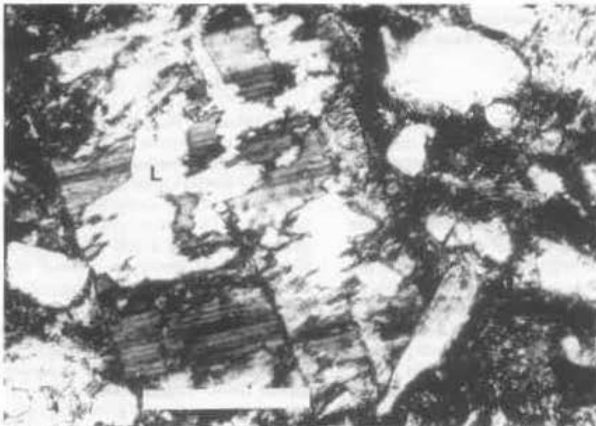
Figure 2.15 White, patchy laumontite (L) (low birefringence) replacing albite-twinned calcic plagioclase in Tyee Mountain turbidite sandstone. Sample RN-91-021, crossed nicols, 10X, scale bar = 0.2 mm.
