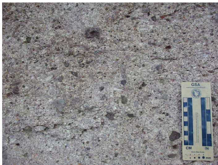
Figure 8. Pumice- and lithic-rich intracaldera tuff exposed at stop 3.
