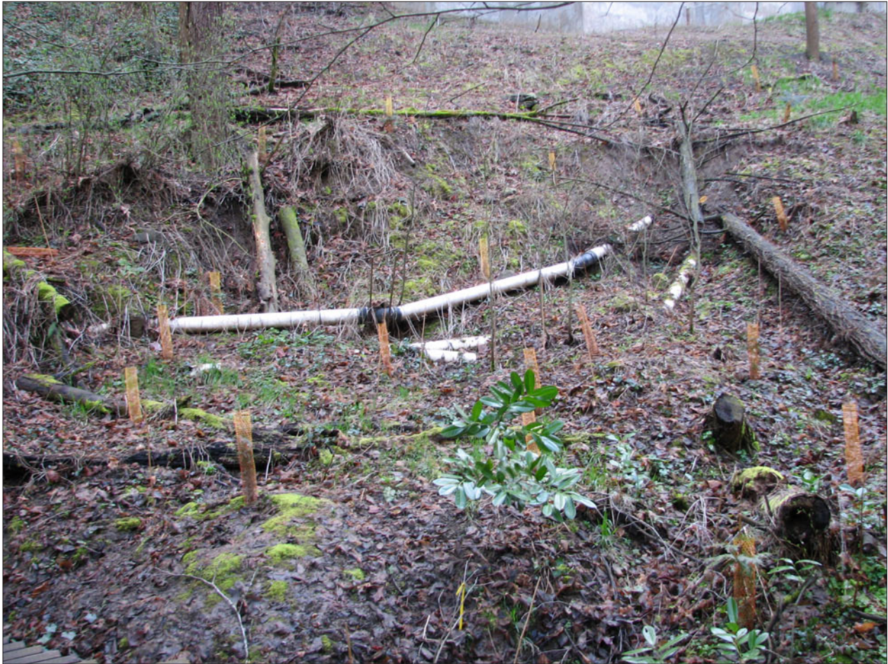
Figure 2-4. Small landslide in Portland Hills Silt along the trail below OHSU. The slide spans about 8 m.
