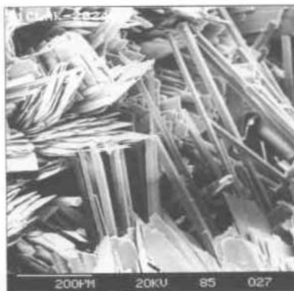
Figure 20. Scanning electron micrograph showing bladed thomsonite and acicular scolecite that fill fractures in a basalt outcrop in the Breitenbush-Austin Hot Springs area.
