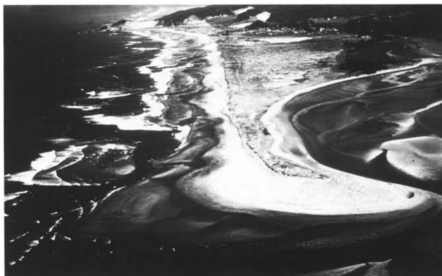
Figure 10. Beach along Nestucca Spit, photographed during low tide, showing troughs and embayments eroded by longshore currents and rip currents.
