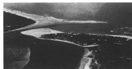
Figure 25. Deflection of channel leading into Alsea Bay by northward growth of longshore bar in response to storm waves related to 1982-83 El Niño and arriving from southwest. From Komar (1986).
