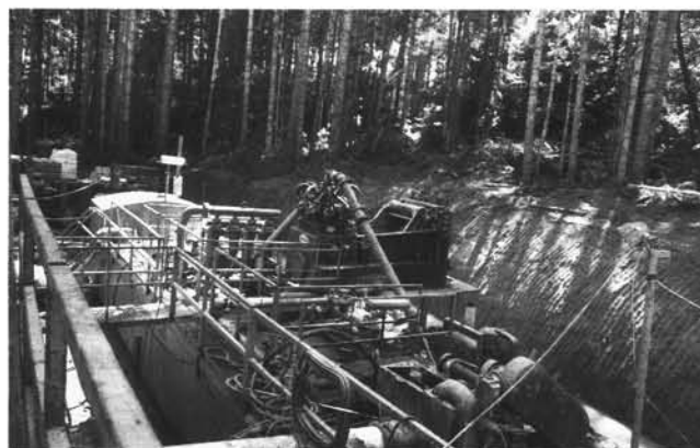
Mud pits at the Nahama and Weagant Energy Company well CC 34-31-65. Mud pits hold the drilling mud that is pumped to the bottom of the drill hole to lift rock cuttings (produced at the bit) to the surface for examination. The drilling mud is also needed to contain the underground pressure that is exerted by the fluids in the rock formation surrounding the hole, to maintain the stability of the well, and to lubricate and cool the drill bit.
