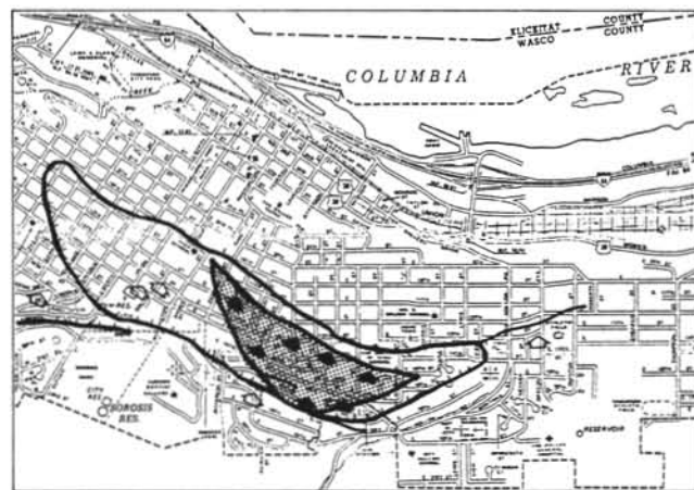
Figure 8. Landslide area in The Dalles. Outlined arrows indicate damage to structures, streets, and utilities due to ground movement; solid arrows indicate recent slide activity. Stippled area shows most active "inner zone" of this nested slide block. Modified from Sholin (1982).
