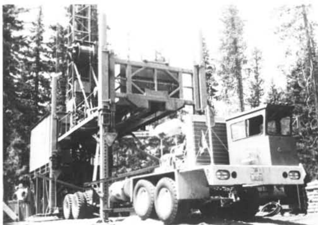
Figure 8. Drill rig used for diamond coring at the Santiam Pass scientific drilling project. Rig was operated by the Tonto Drilling Company and is capable of drilling to 1.2 km. Drilling from 141 m to 928 m took 35 days starting August 14, 1990.
