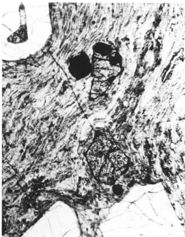
Figure 2. Photomicrograph of densely welded tuff along the North Fork Winberry Creek (sample 1, Table 1, plane-polarized light). Eutaxitic texture is defined by flattened and deformed glass shards. Two clinopyroxene grains are near center of photo; the one containing opaque grains is about 0.3 mm in long dimension. Three large plagioclase grains are near edges of photo.
