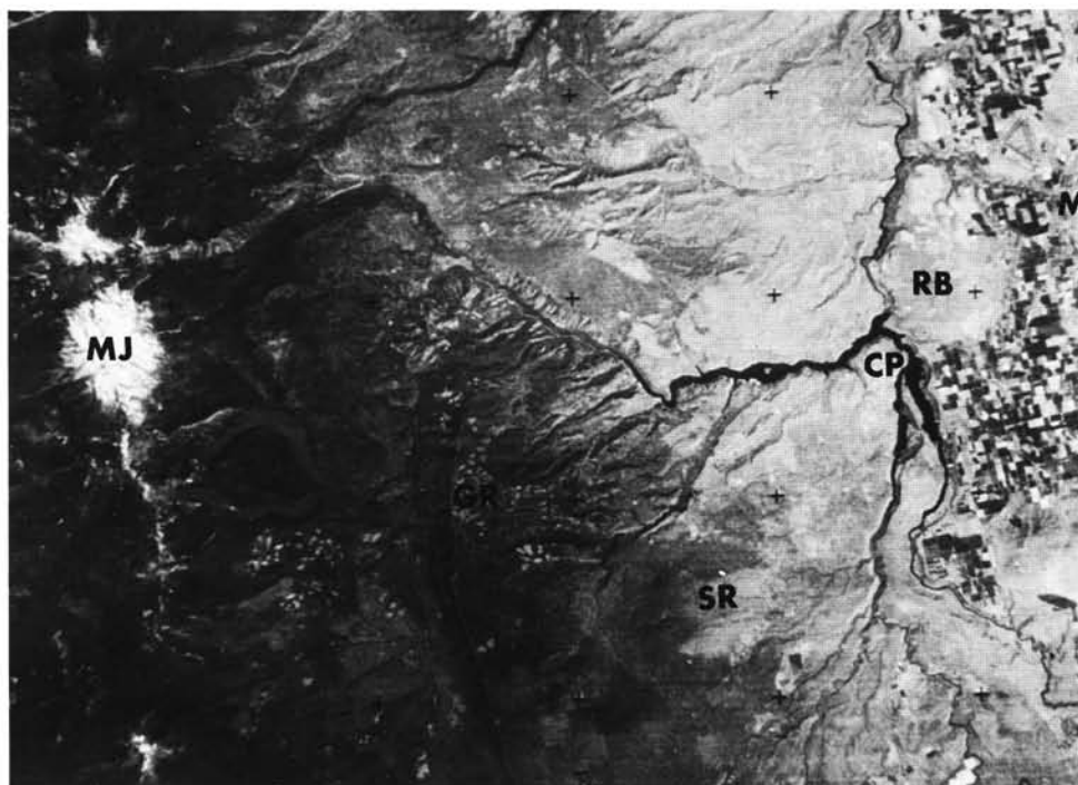
Figure 2. Landsat RBV image of part of central Oregon showing the High Cascade Range on the west and Deschutes basin on the east; crosses are spaced at approximately 10-km intervals. MJ= Mount Jefferson; GR= Green Ridge fault escarpment; SR= Squawback Ridge, late Pliocene shield volcano; CP= The Cove Palisades State Park marking the confluence of (clockwise from upper left) the Metolius, Crooked, and Deschutes Rivers; RB= Round Butte, early Pliocene shield volcano; M= Madras.
