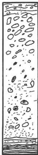
Figure 19. An ignimbrite section, typical of those in the Deschutes Formation. After Sparks and others (1973).
