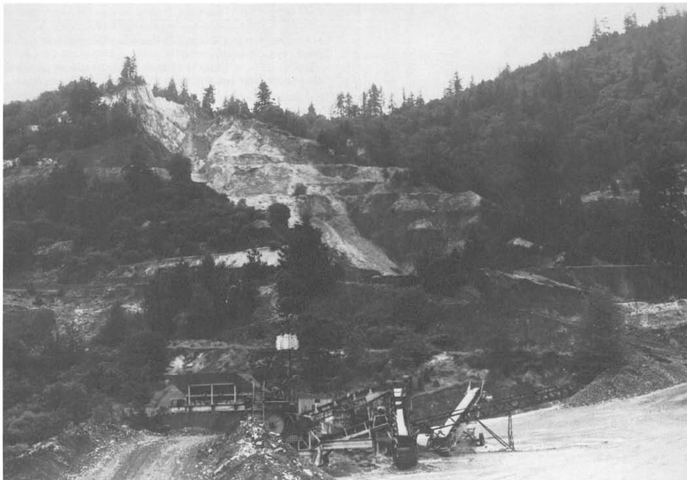
Figure 3. Bristol Silica and Limestone Company: silica quarry and primary crusher. Dolomite occurs along the upper left edge of the quarry (Figure 2, active mine site 21).
