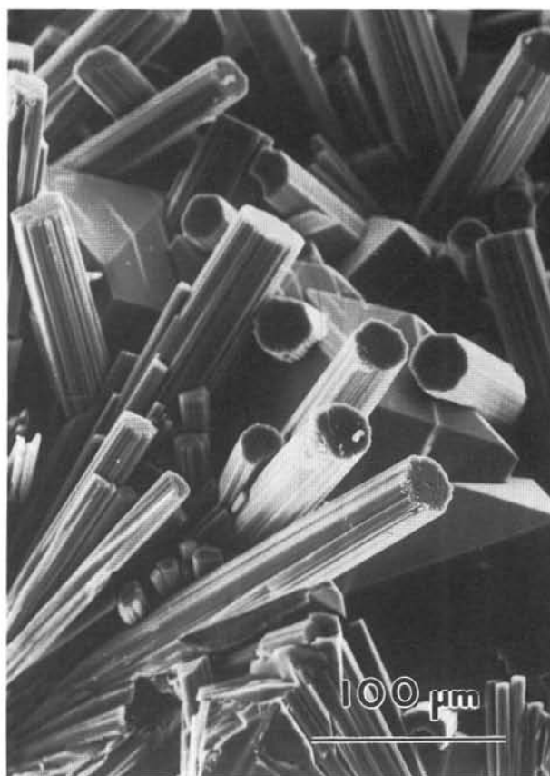
Figure 12. Scanning electron micrograph showing columnar bundles of erionite crystals and later blocky heulandite crystals from 887-m depth.
