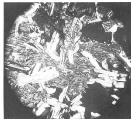
Figure 10. Photomicrograph of diktytaxitic basalt. Note rectangular, lathlike plagioclase crystals protruding into cavities. Photo courtesy of Marvin Beeson.
