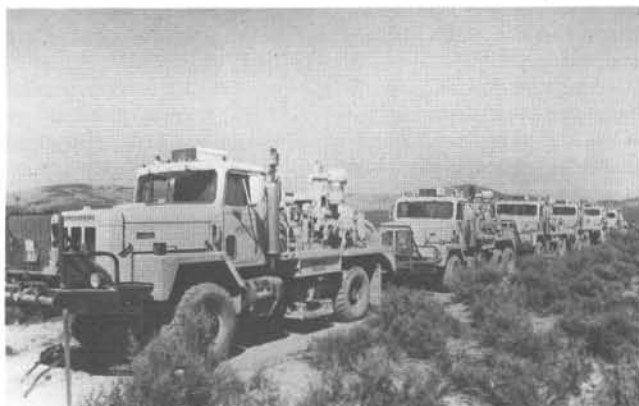
Specially designed vibrator pads located beneath the trucks are vibrated to create sound waves for the vibrating energy source method of exploration.
