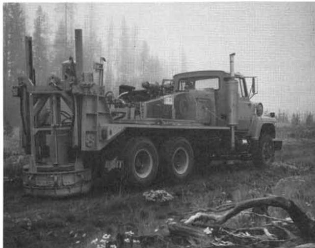
An air gun using compressed air inside a bag filled with water is mounted on this truck and discharged to generate seismic sound waves.
