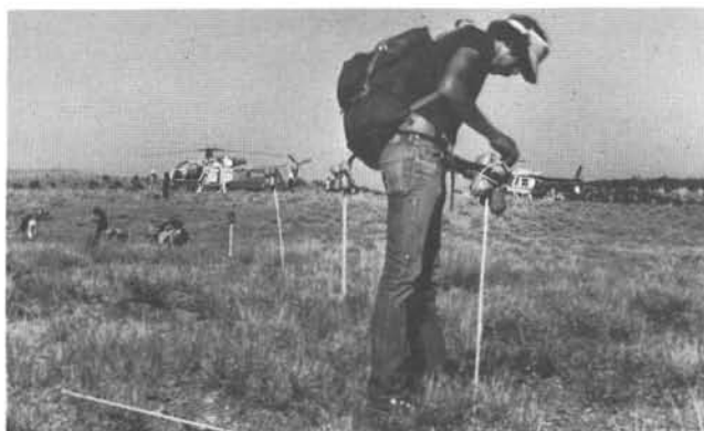
Explosive charges for surface detonation are mounted on wooden stakes above the ground.
