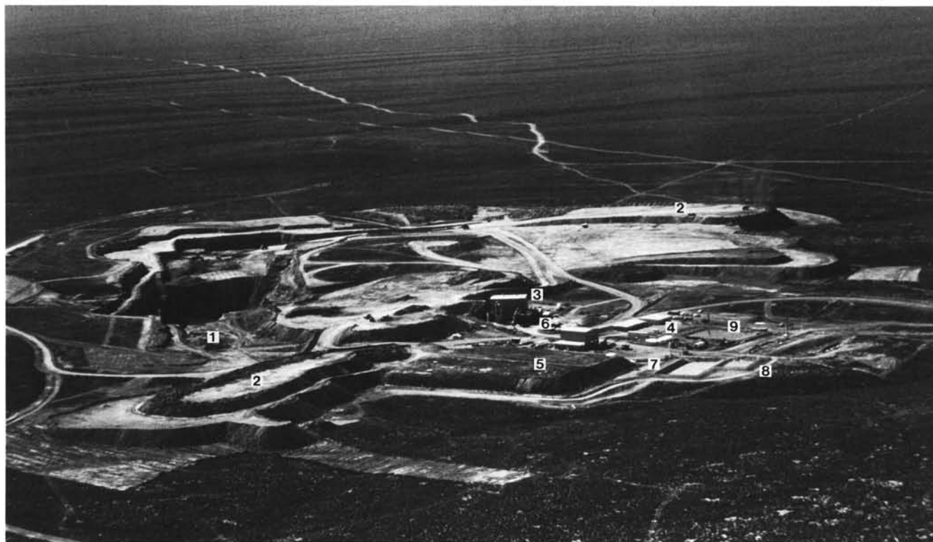
Aerial view of gold mine and processing facilities of Atlas Gold Mining, Inc., in Eureka, Nevada. 1=open-pit mine; 2=waste dumps; 3=crusher and mill; 4=administration, laboratory, and maintenance buildings; 5=heap leaching pad; 6=carbon columns; 7=pregnant pond; 8=barren pond; 9=fresh-water pond. Photo courtesy of Atlas Gold Mining, Inc.
