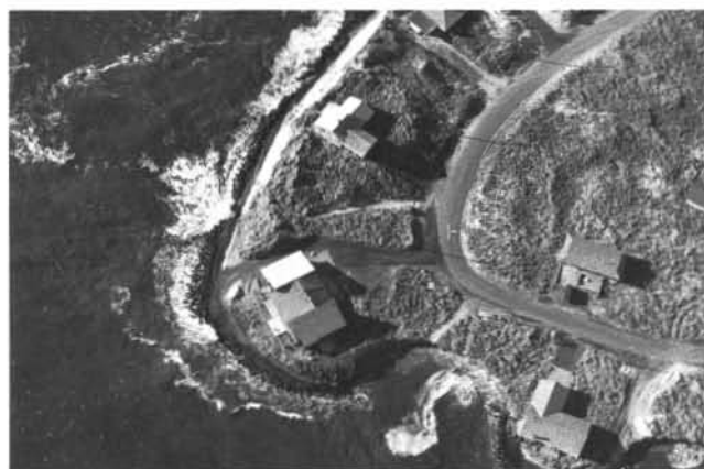
Swirling tidal eddies gouge erosional cusps along the tip of Alsea Spit, while homeowners battle the severe loss of property with basalt riprap.
