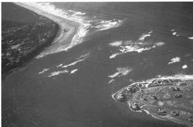
By December 1985, the Alsea Bay inlet had widened to its maximum extent. Homes on the spit protected by rock revetments were isolated on peninsulas between unprotected vacant lots.
