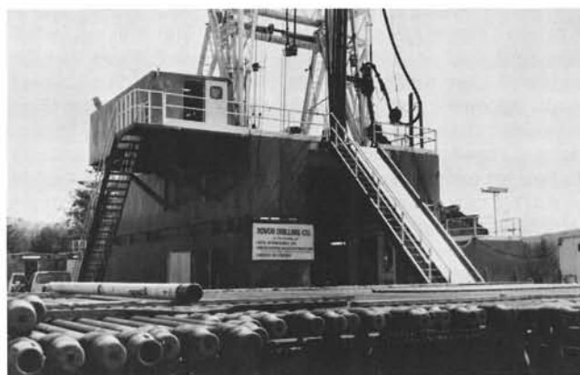
Base and pipe racks of new ROVOR drilling rig.
