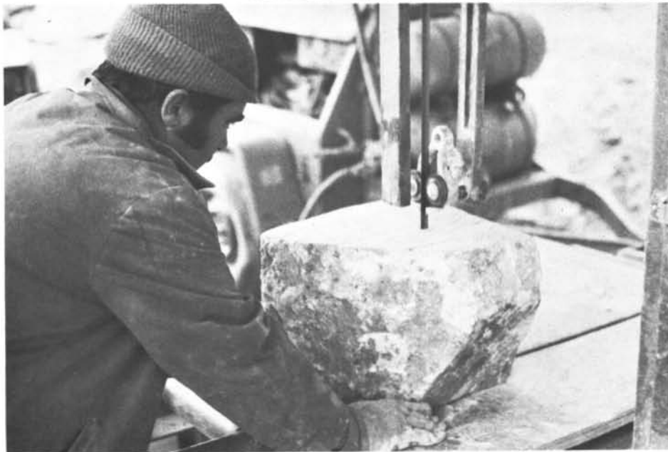
Figure 9. Soapstone is soft enough to be trimmed by chain saw, band saw, or other saw with specially hardened teeth. Here it is being cut with a special gang saw into specific sizes for marketing.
