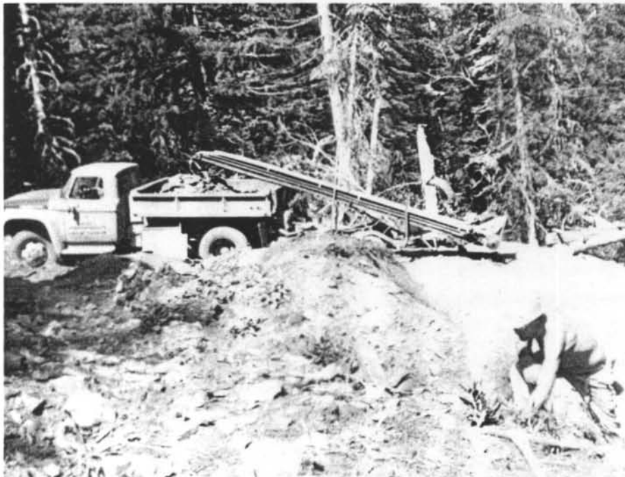
Figure 13b. Small-scale mining operation at Cone Peak emery deposit. Only mechanical equipment used is gasoline-driven conveyer and dump truck.
