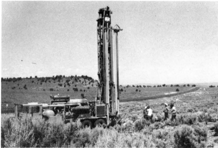
Department's drilling project to measure heat flow along the Brothers fault zone in Harney County, central Oregon. Measurement of heat flow patterns in this area of young volcanic rocks assists in regional evaluation of potential geothermal energy resources.
