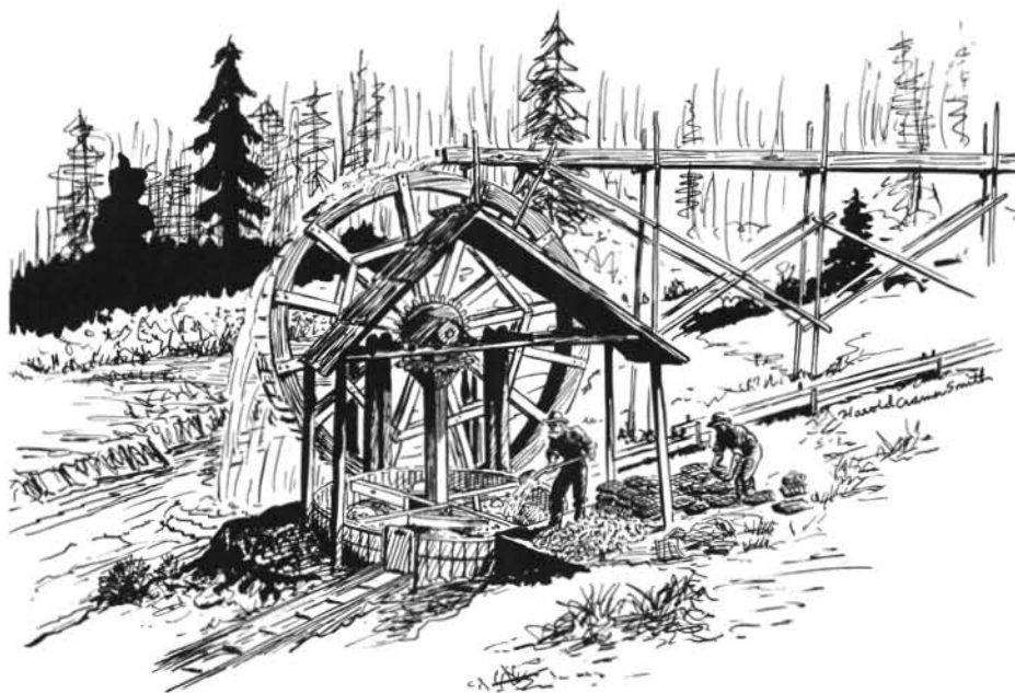
Figure 5. Arrastre used to grind friable gold and silver ore. Ore spread on floor was crushed by heavy stones chained to arms pivoting around central shaft. In this drawing, water provides power to turn shaft; in other cases, horses or steam could be used. Gold was then recovered, as it was from a stamp mill, by sluicibox and copper-mercury-coated plate.
