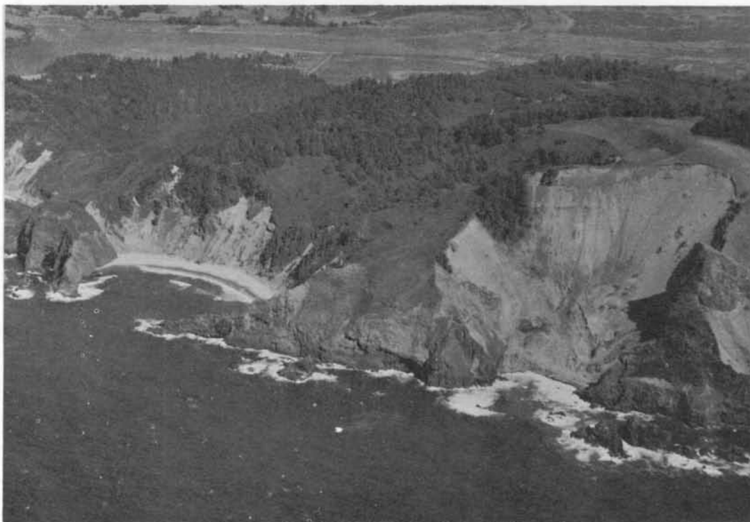
Figure 6. Slumping of Eocene shale south of the Salmon River. Where basalt cap has been breached, landsliding has been most rapid.
