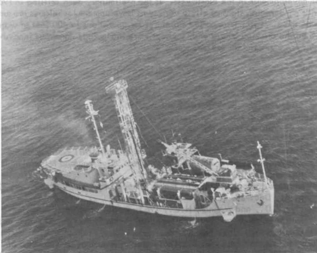
Caldrill I. (Caldrill Offshore, Inc.) A center-well core-drilling ship used by Standard Oil Co. and Union Oil Co. to drill shallow core holes off the Oregon coast in 1964. Large outboard motors position the vessel, so that no anchors are needed during the drilling operation..
