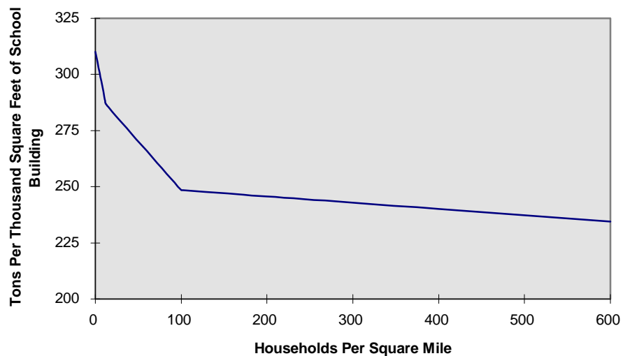
Figure Chapter Two -11 Aggregate Usage Rates Versus Household Densities for Western Oregon School Construction
