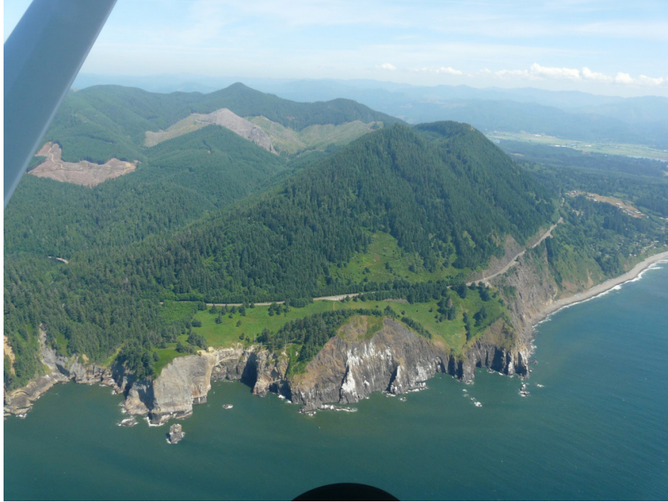
Figure 2-5. View is looking east toward Neahkahnie Mountain. U.S. Highway 101 can be seen around mid photo tracking along the mountain. To the right and along the toe of the cliff is an extensive gravel/boulder berm that has formed as a result of rockfalls and landslides off the headland. (Photo: L. Stimely, DOGAMI, 2011)
