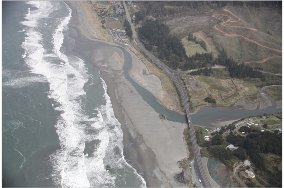
Figure 15. In early spring 2010, Hunter Creek migrated so far northward that it began to erode the toe of several homes constructed immediately adjacent to the creek and beach. Note the locations of at least two of the groynes, which are depicted by the two prominent horns at the back of the beach around mid-photo. (Photo taken on April 9, 2011; courtesy of Ron Sonnevill, geotechnical consultant, Terraforma Building, Inc.)
