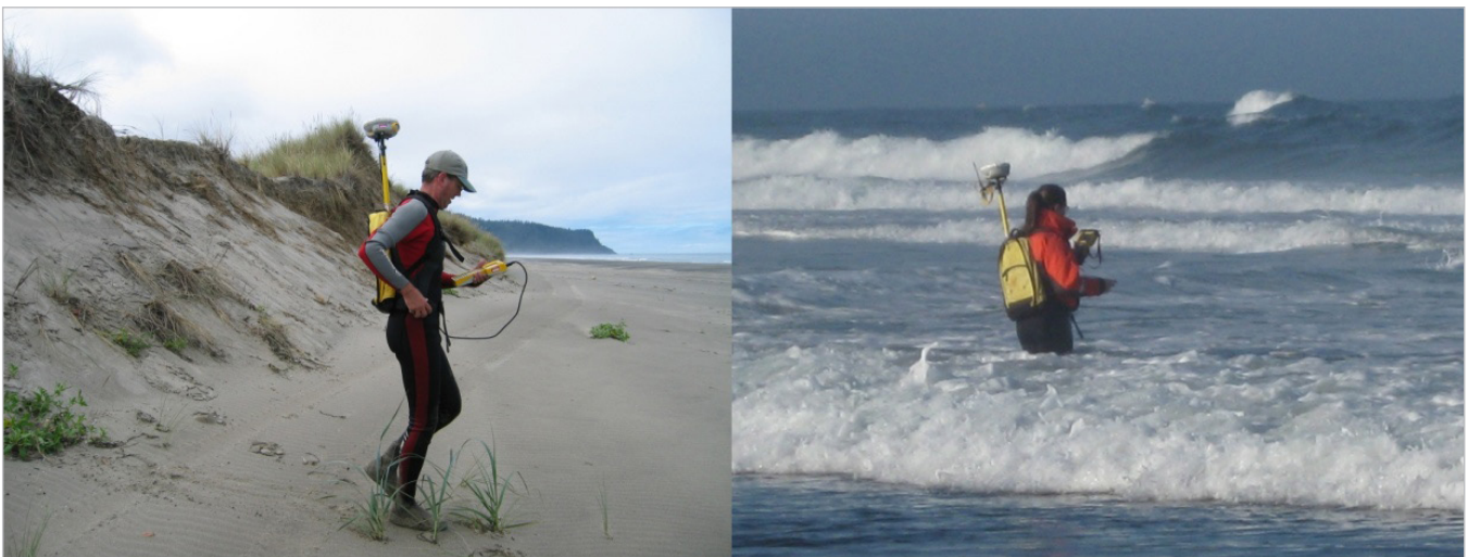
Figure 10. Beach profile surveys being undertaken using a Trimble R8 GPS rover mounted on a backpack.
