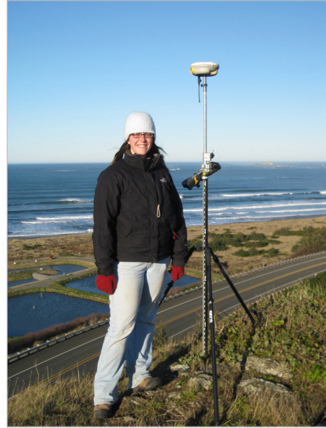
Figure 9. Static GPS occupations were used as part of a site calibration on selected benchmarks to derive a local coordinate system in the Gold Beach and Netarts area. GPS site calibration procedures involved occupying a benchmark for 180 epochs (typically at least 3 minutes or longer) and then processing the data in Trimble Business Center (TBC) software. Example here is of the Trimble R8 receiver located on National Geodetic Survey monument OA0832 just north of the Rogue River, with geologist Laura Stimely standing by.
