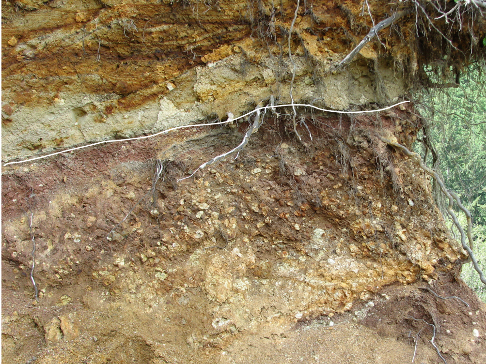
Figure 5. Failure plane in Dutch Canyon landslide complex (unit Plld). Photo looking northeast from station PDX-1146 (NAD 83 UTM coordinates 507,085 m E and 5,062,719 m N) shows tan-white Scappoose Formation sandstone thrust (white line) over red-brown paleosol developed on top of Columbia River Basalt Group.
