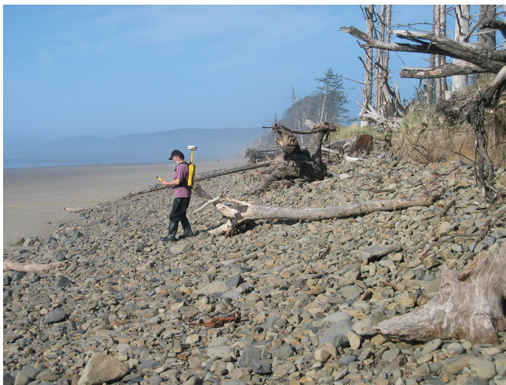
Figure 5. Beach surveys were undertaken by walking lines perpendicular to the waters edge, navigating along a predetermined line identified on a hand-held TSCe Trimble computer, connected to the Trimble 5800 GPS rover. Example here is of R. Hart undertaking a profile survey of the beach at Cape Lookout State Park.
