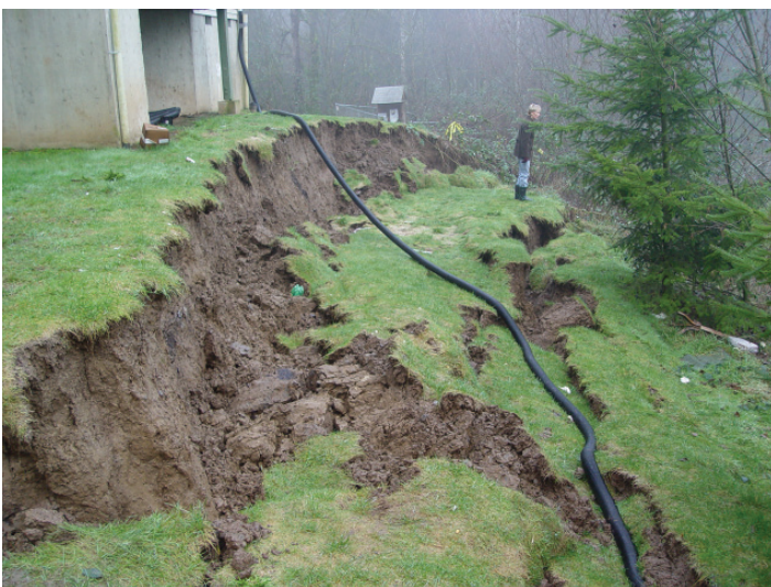
Figure 8. Photographs showing scarps along the crest of the toe of the large Newell Creek Apartment landslide from (left) 2006 and (right) 2007.
