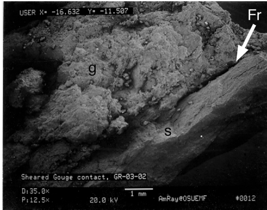
Figure 5B. SEM photomicrograph at low magnification (12.5X) shows a sharp smooth shear plane (labeled Fr) which appears to step across the specimen. The specimen was mounted upside-down which places the shear gouge (g) in the upper NW half of the photograph and the unsheared siltstone (s) in the lower SE half of the photograph. The sheared gouge appears as a jumbled mass of largely subparallel (imbricated) smectite clay particles or packets. In the gouge, multiple fractures (dark lines), along which slippage has occurred, subparallel the main shear boundary.
