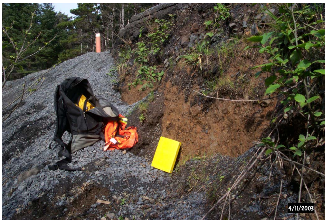
Figure 13. Sites JC-22 (near red highway cone at top of highway embankment) to JC-24 (to the right of the yellow field book) looking northeast parallel to the strike of the fresh headscarp (red orange fill of excavated Astoria Formation). Yellow field book is ~19 cm long. Near vertical portion of scarp is ~1.2 m high.
