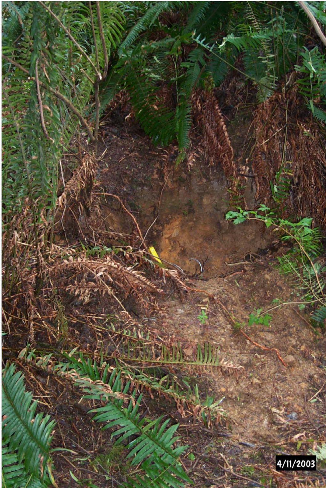
Figure 10. .JC-20 site looking south. Yellow field book is ~19 cm long. Scarp cuts Old Coast Highway. The scarp is in weathered Astoria Formation colluvium below the Old Coast Highway and some gravel fill from the adjacent private driveway.
