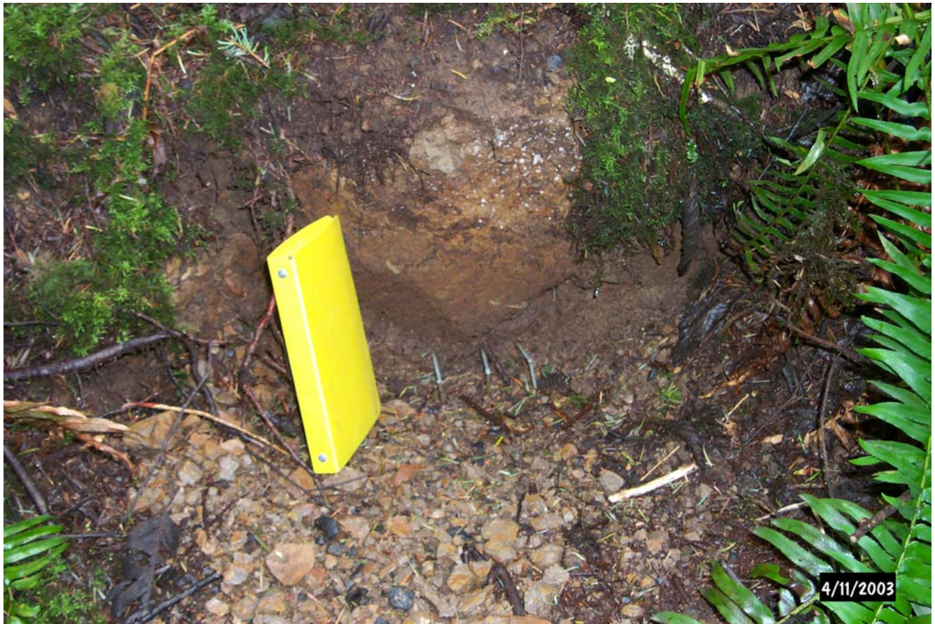
Figure 9. JC-19 location looking south. Yellow field book is ~19 cm long. Note that all nail heads are still touching in this April photograph, so no significant movement occurred. Scarp is in relatively fresh Astoria Formation siltstone and sandstone with a thin covering of gravel from the Old Coast Highway.
