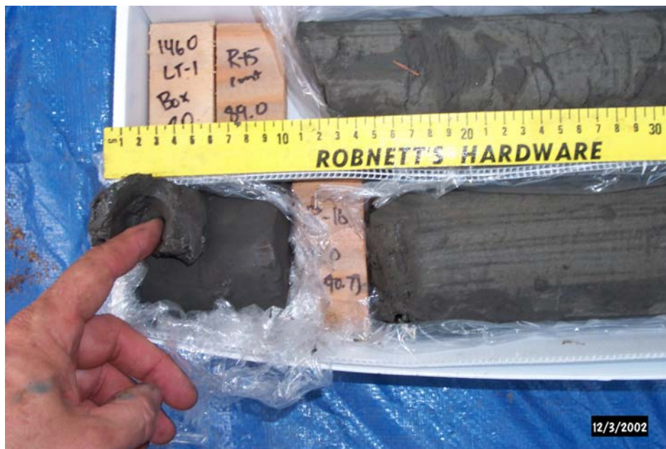
Figure 14. Soft wet silty gouge at slide plane in borehole LT-1 at 27.4 m (90 ft) depth.
