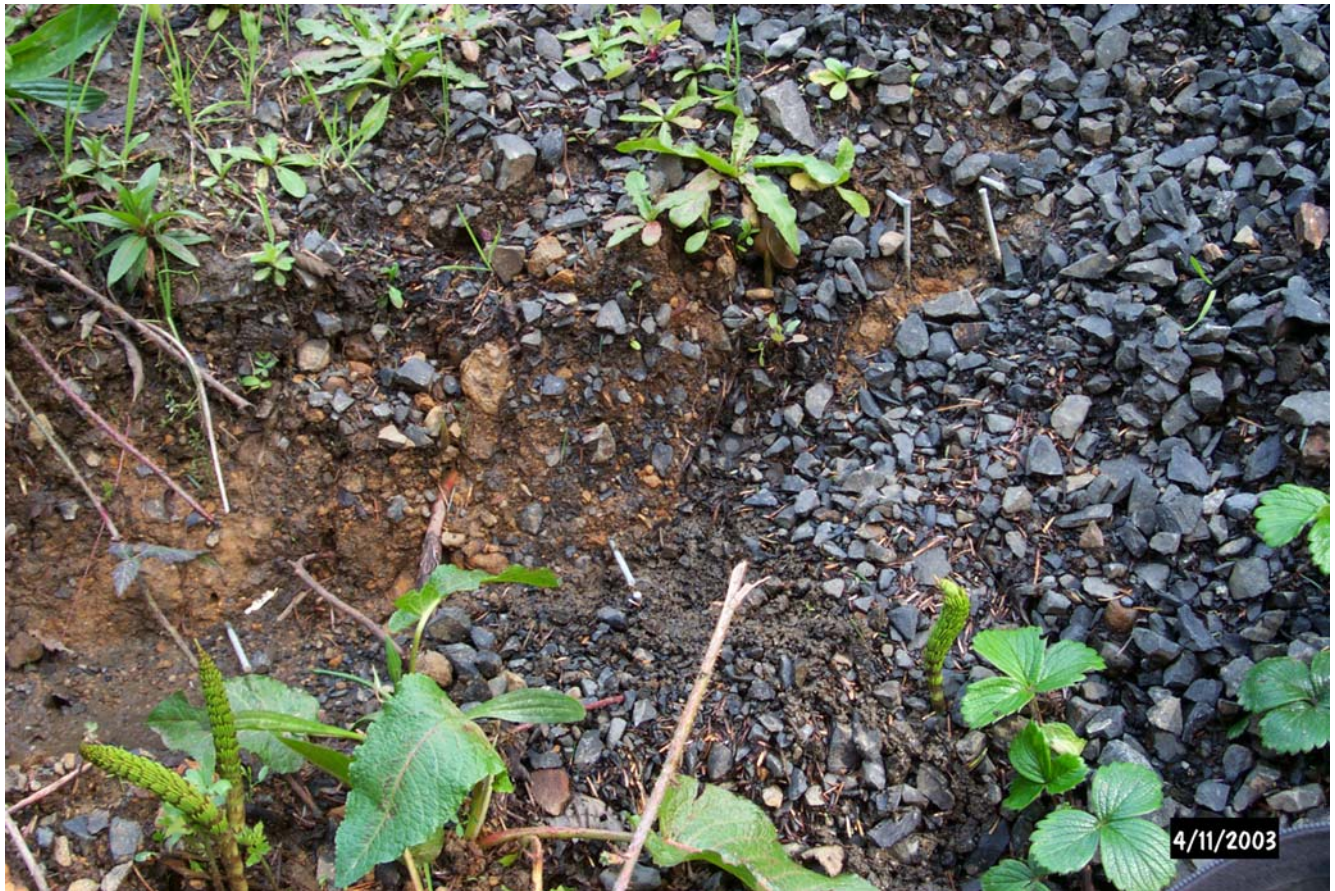
Figure 8. JC-18 site, looking southeast. The scarp is in gravel fill from the forest road. Exposed portions of the two vertical nails is on the right~1.2 cm long. Note that fresh gravel dumped on the road has disturbed the nails on the right, so that measurement was not used.
