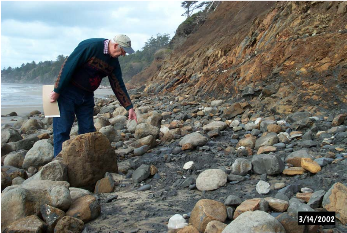
Figure 4. Highly sheared dark gray sandy siltstone unit at the toe of the Johnson Creek Landslide. Chuck Dennison of Dennison Surveying is pointing at the soft, highly deformed material.
