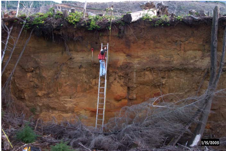
Figure 5. Pleistocene marine terrace sand exposed in the northeast headwall of the landslide. Jonathan Allan of DOGAMI is measuring the thickness of the unit. Note the nearly flat surface of the sand sheet. The contact with underlying Tertiary Astoria Formation is ~1 m below the base of the ladder.
