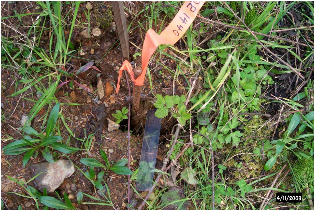
Figure 6. JC-17 site with displaced steel survey marker at headscarp, looking east. This stake was not used in the resurvey.
