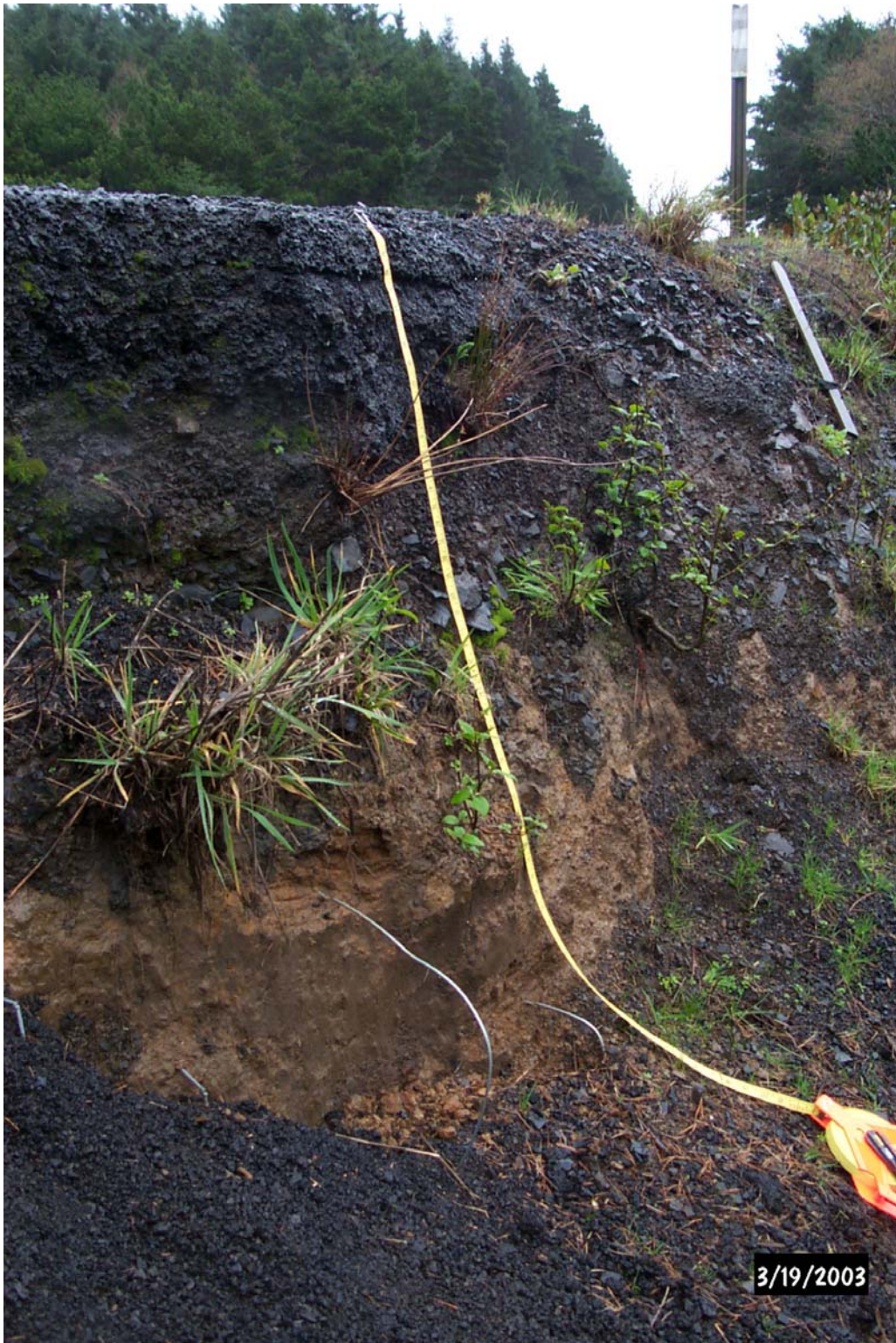
Figure 15. JC-23 site with both wires and nails, looking south southeast. Scarp is in red orange fill of excavated Astoria Formation overlain by gravel and asphalt. Near vertical portion of scarp is ~1.2 m high.
