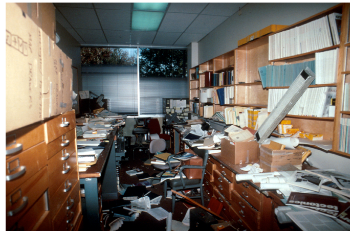
Even without structural damage, offices like this one after the 1989 Loma Prieta, California earthquake may be a mess with overturned bookcases, filing cabinets and desks. The safest way to protect yourself is get under a desk or table. DO NOT stand in a doorway. Photo: J. K. Nakata, USGS
