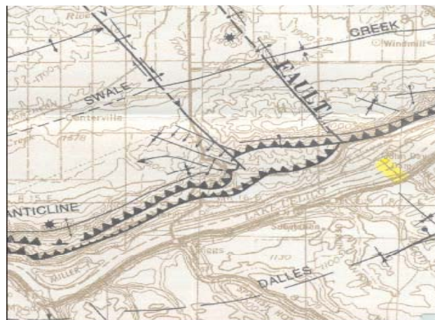
Figure 8.8. Neotectonics in the John Day Lock and Dam area showing nearby active fault structures. The dam is located to the right of the center (source: Bela, 1982).
