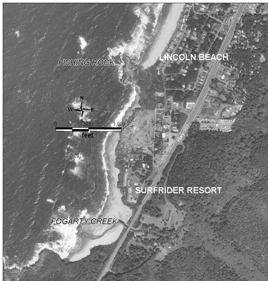
Figure 1 Location of Surfrider Resort. North-south trending portion of sea cliff is area of concern. Note the gap in offshore rocks immediately west of the resort that allow waves to break much closer to the beach.
