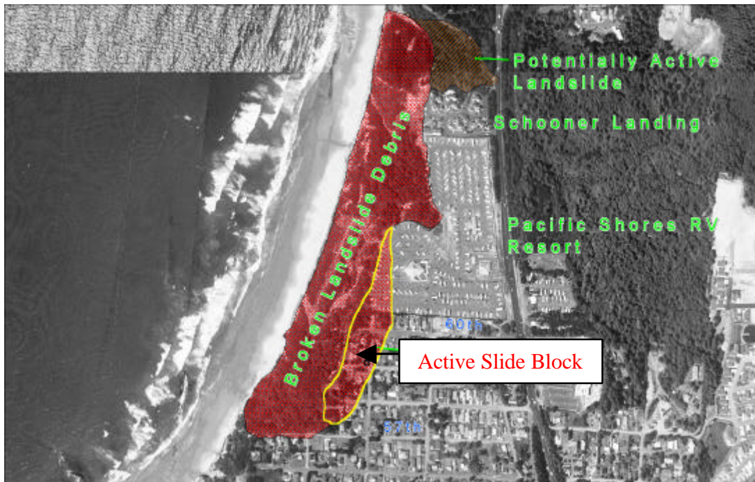
Figure A 1 Schooner Creek landslide of Newport, Oregon showing an active slide block that has begun to displace city streets over the last few decades but has only a few feet of lateral and vertical displacement. Meanwhile, the broken landslide debris in front of this block continues to move seaward in response to wave erosion and high groundwater, opening up fissures in front of the block. Movement on the active block has apparently ceased from about May of 2000 to present (June, 2001). This period has been characterized by unusually low rainfall on the Oregon coast.
