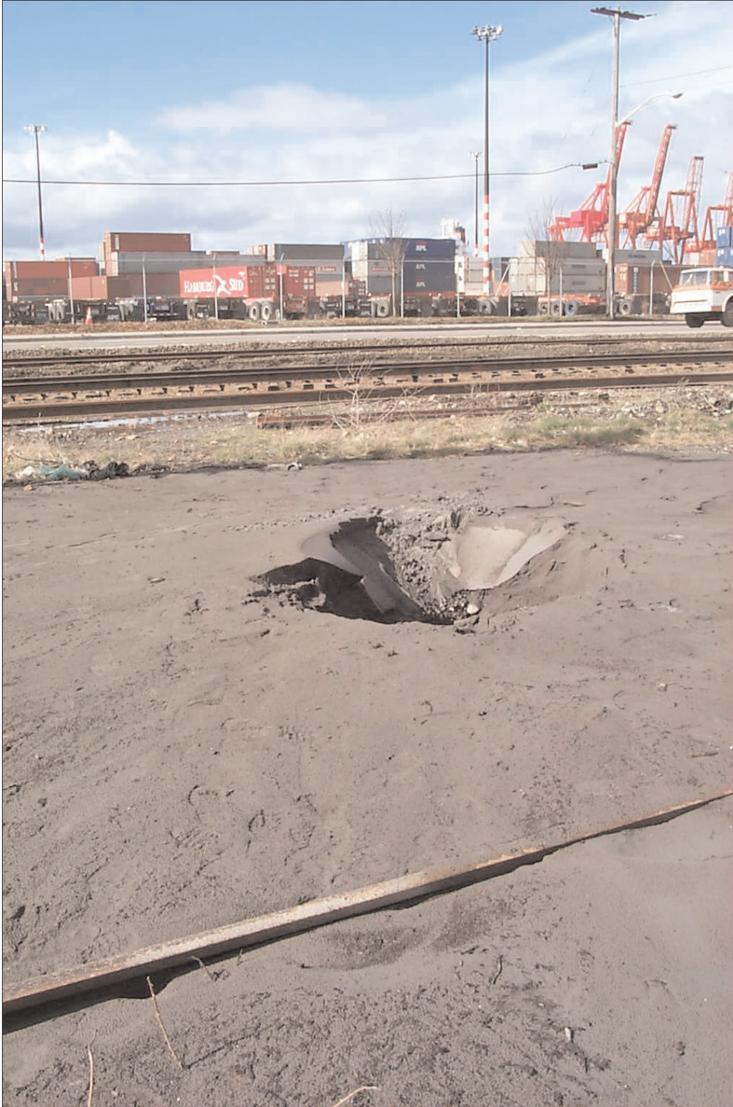
Photo 10. Sand boil along railroad tracks paralleling E Marginal Way in Seattle – Terminal 30 in the background.
