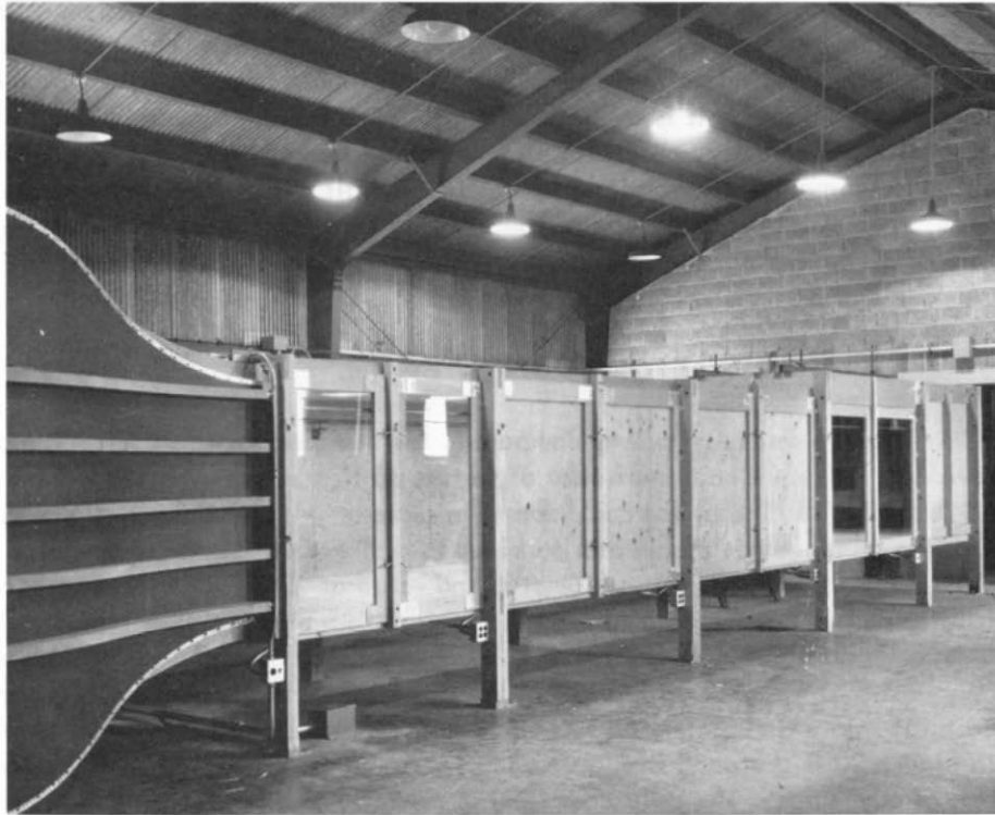
Figure 18. Wind tunnel to be used with models as an aid in site selection and in testing models of aerogenerators of various types.
