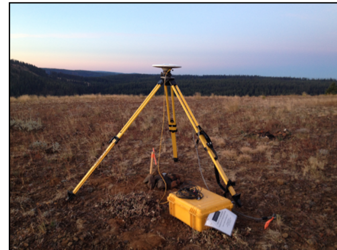
Trimble R7 Receiver set up over GPS monument "UMA_2"
