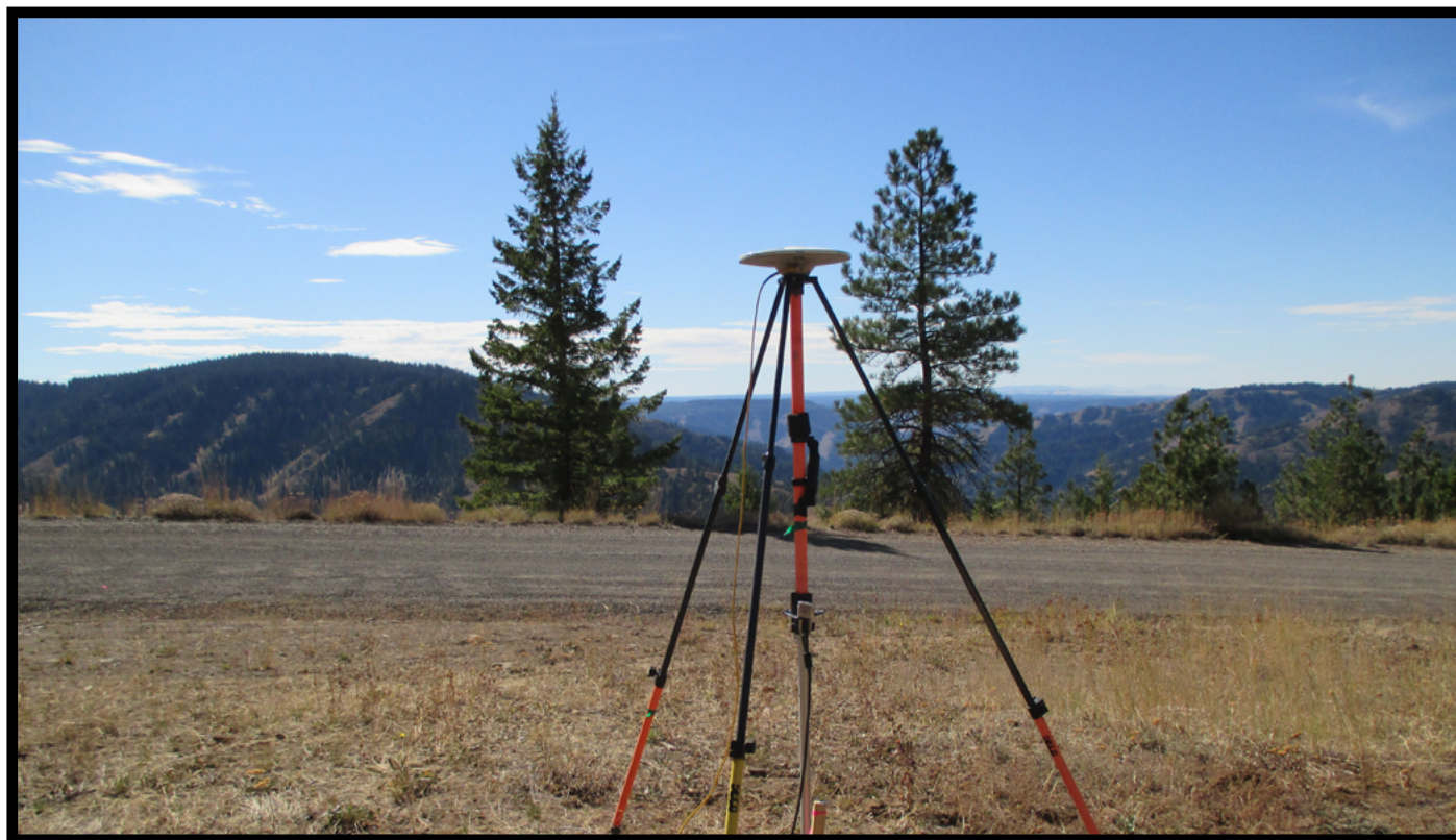
Trimble R7 set up over GPS Monument "UMA-03"
