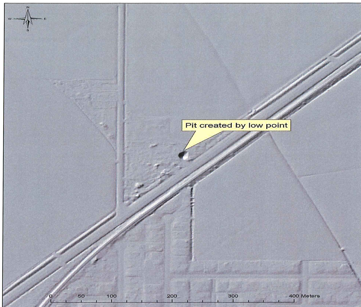
Figure 7. Example of “Pit” caused by low point in ground model. Pits are caused when standing water absorbs the lidar pulse. Pits are evident in ground model as the lowest point elevation is assigned to the grid cell value. Inversely the pit is not observable in the highest hit model as the highest point elevation is assigned to the grid value.
