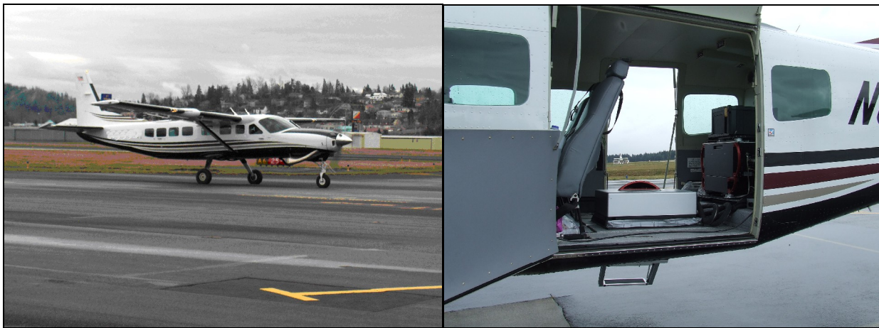
The Cessna Caravan is a powerful, stable platform, which is ideal for the often remote and mountainous terrain found in the Pacific Northwest. The Leica ALS50 sensor head installed in the Caravan is shown on the right.
