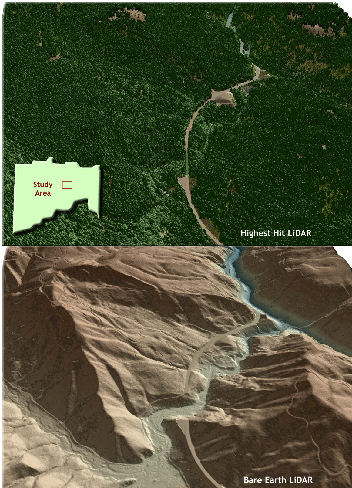
Figure 7.15. 3-d oblique view of LiDAR-derived surfaces showing an historic landslide along Devils Lake Fork, between Elliot Creek and Drift Creek.
