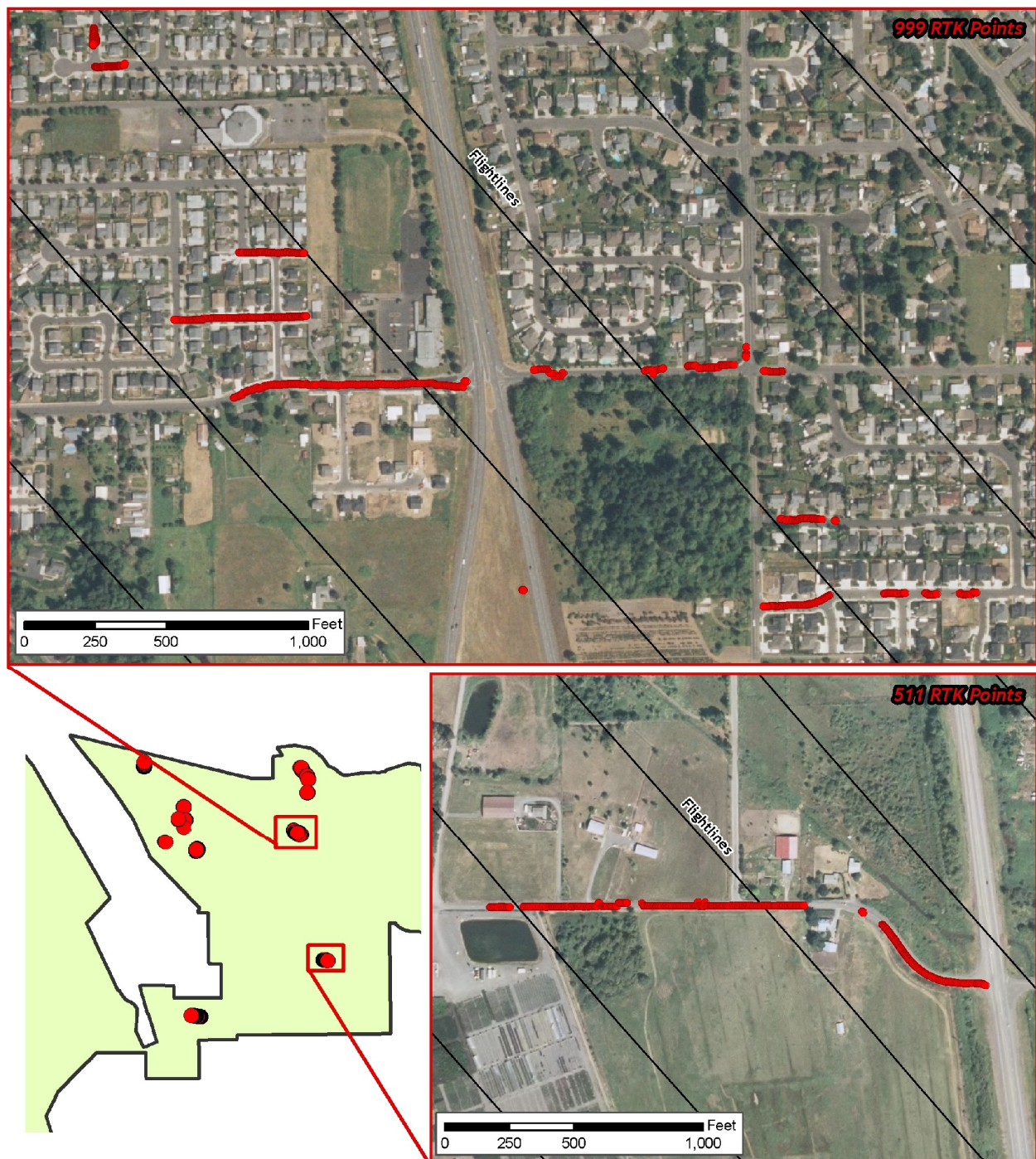
Figure 2.12. RTK point locations in the DOGAMI study areas; color images are NAIP Orthoimages.
