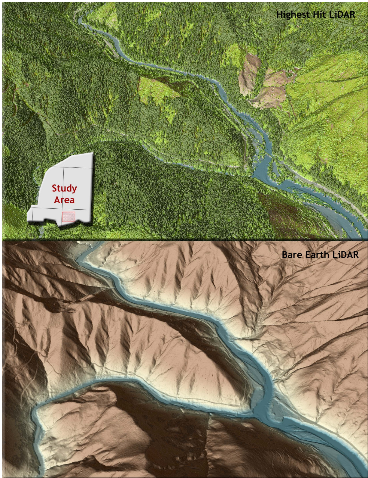
Figure 7.10. 3-d oblique view of LiDAR-derived surfaces in 7.5' Quad 45123D6, showing the confluence of the Wilson and Little North Fork Rivers in the ODF South study area.
