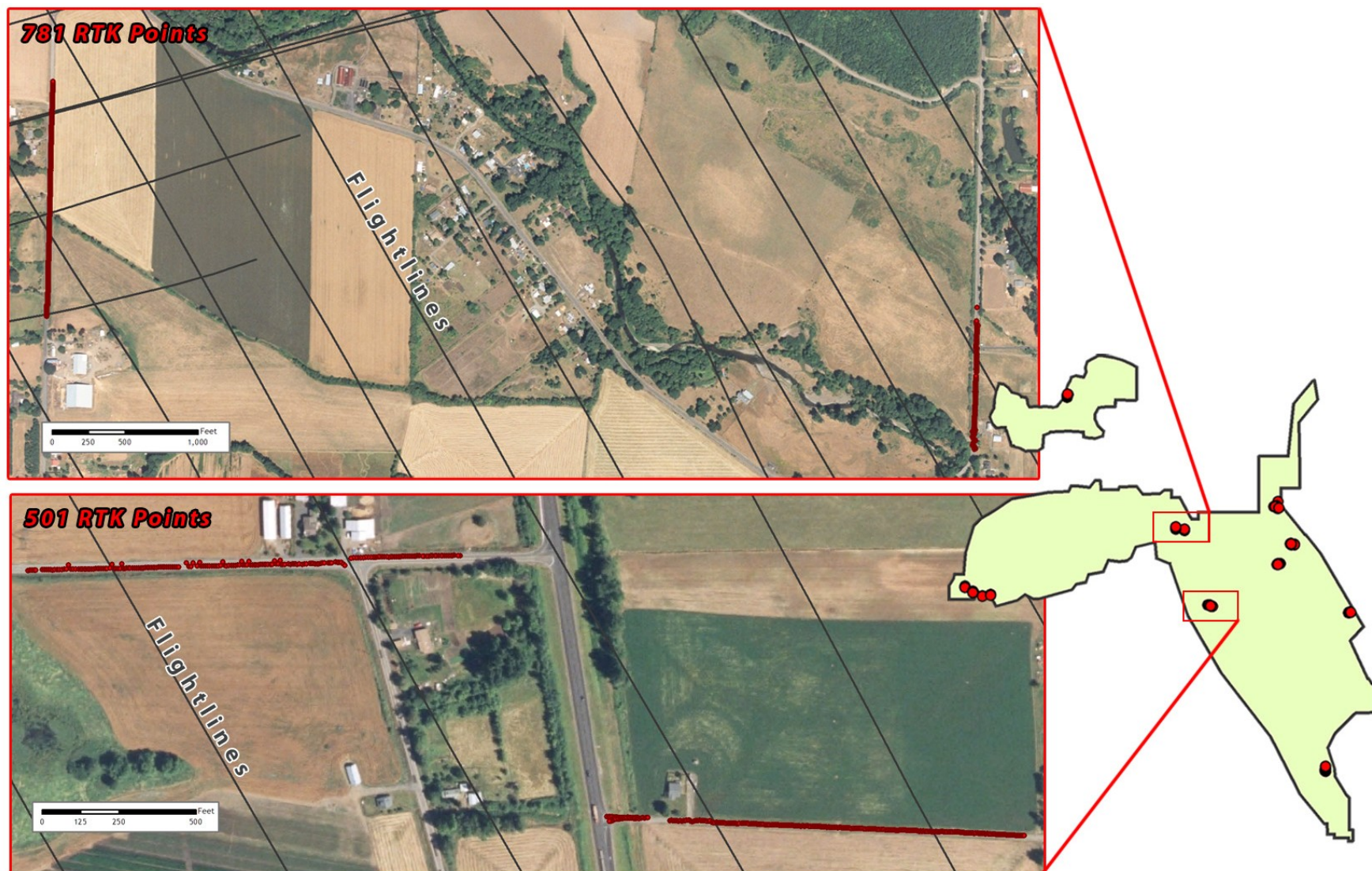
Figure 2.7. RTK point locations in the DOGAMI study areas; color images are NAIP Orthoimages.
