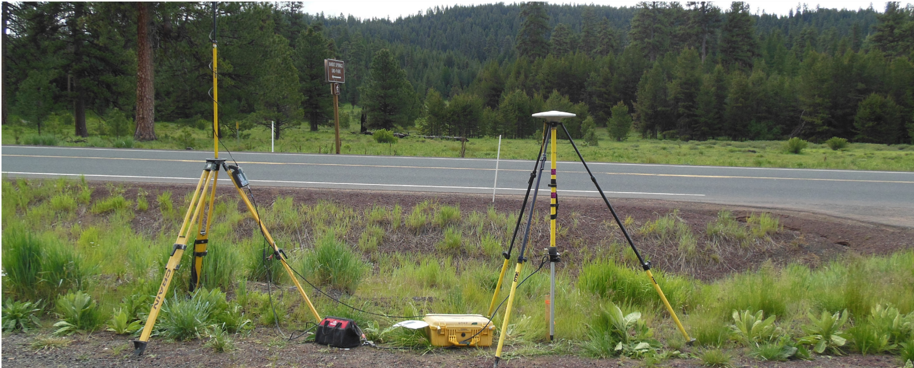
Base station and radio unit set up over control "OCH_02"
