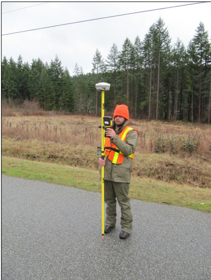
Field ground professional collecting RTK
